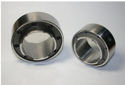
Figure 10.2 Two machined cast bearings of \text{Co}_{1.5}\text{CrFeNi}_{1.5}\text{Ti}_{0.5} HEA made by lost-wax cast method. The outer diameter is 56 mm and inner diameter is 38 mm.
