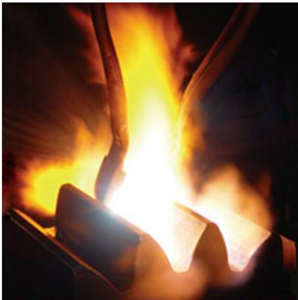
Figure 2-2 — Typical flame hardening.
