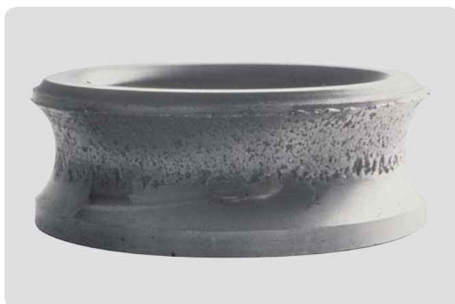
Deep groove ball bearing inner ring Excessive axial load, resulting in too thin lubricant film and surface distress
