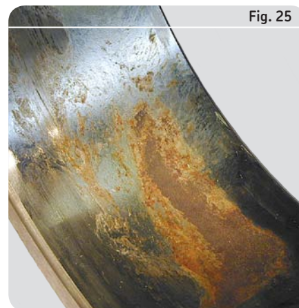
Fretting corrosion on an inner ring bore resulting from heavy load or inadequate shaft seat
