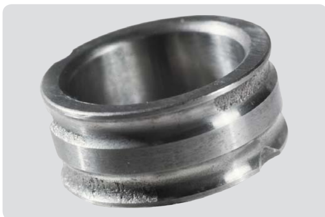
Double row angular contact ball bearing inner ring Excessive misalignment, resulting in excessive loads, with two load zones 180° apart.
