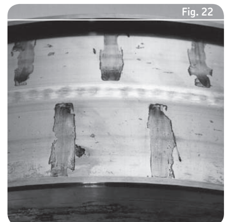
Initial patches of etching at rolling element pitch on the inner ring raceways of a spherical roller bearing
