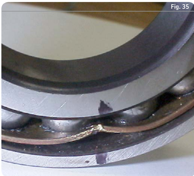
Plastic deformation on the cage of an angular contact ball bearing resulting from poor handling
