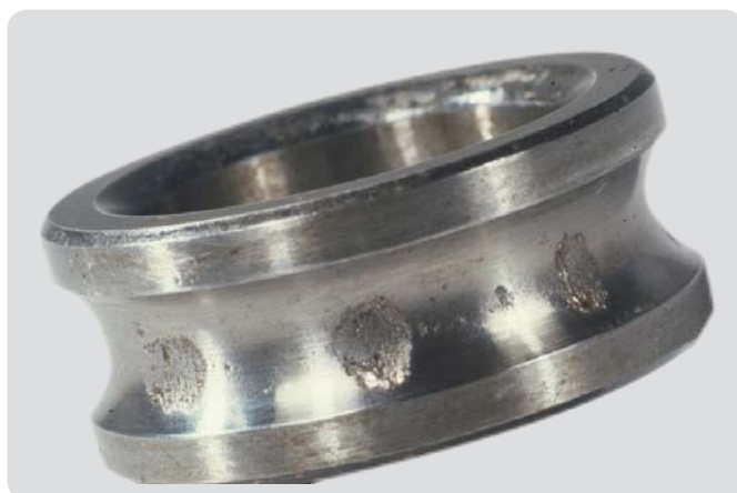
Deep groove ball bearing inner ring Impact during mounting, resulting in spalling at ball pitch
