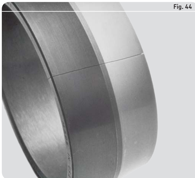
Fractured inner ring of a spherical roller bearing with a tapered bore resulting from excessive drive-up
