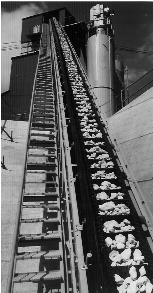
Figure 10.4 Example of pocket belt partitions.
