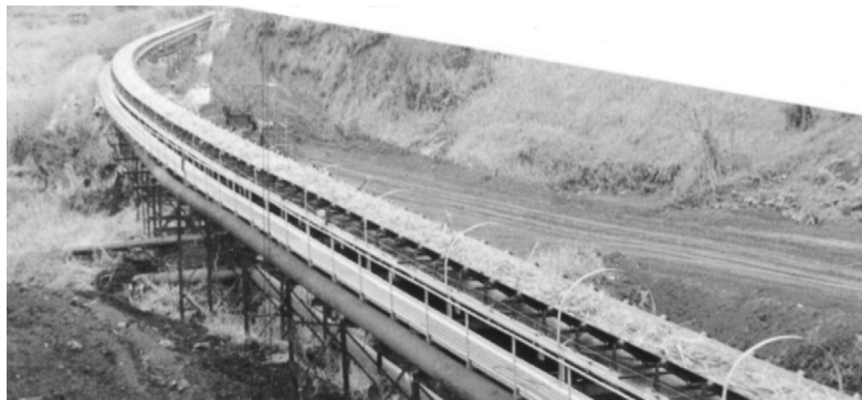
Figure 1.5 Horizontal curve conveyor, conveying following natural terrain.
