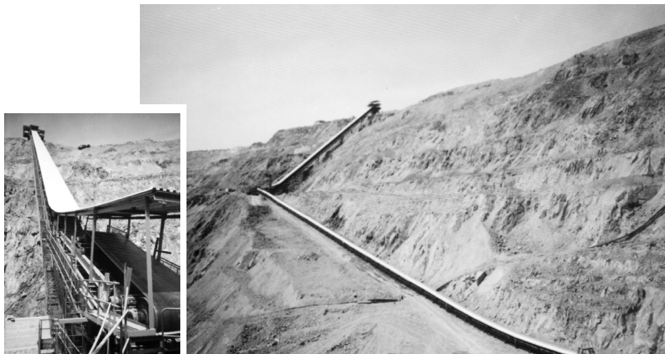
Figure 10.15 Sandwich belt in an open pit mining application.
