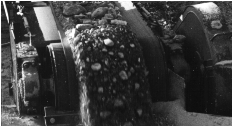
Figure 1.9 Material discharging over conveyor head pulley.
