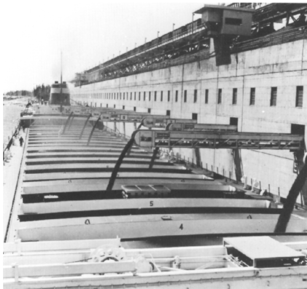
Figure 1.13 Shuttle belt conveyors load and trim taconite pellets onto ore vessel on Great Lakes.
