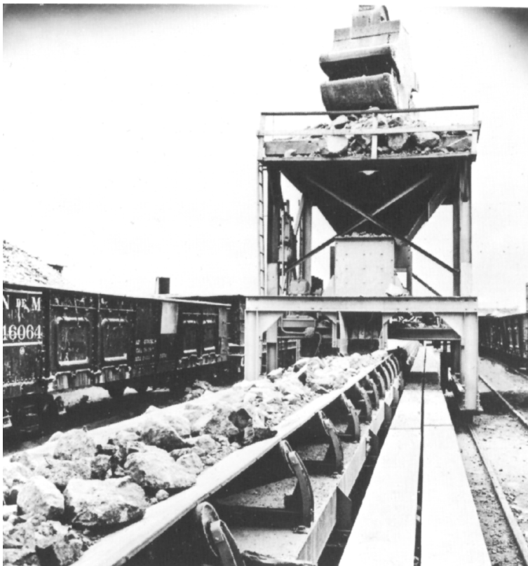
Figure 1.6 Multiple loading stations feed ore to slope conveyor in open-pit mine.
