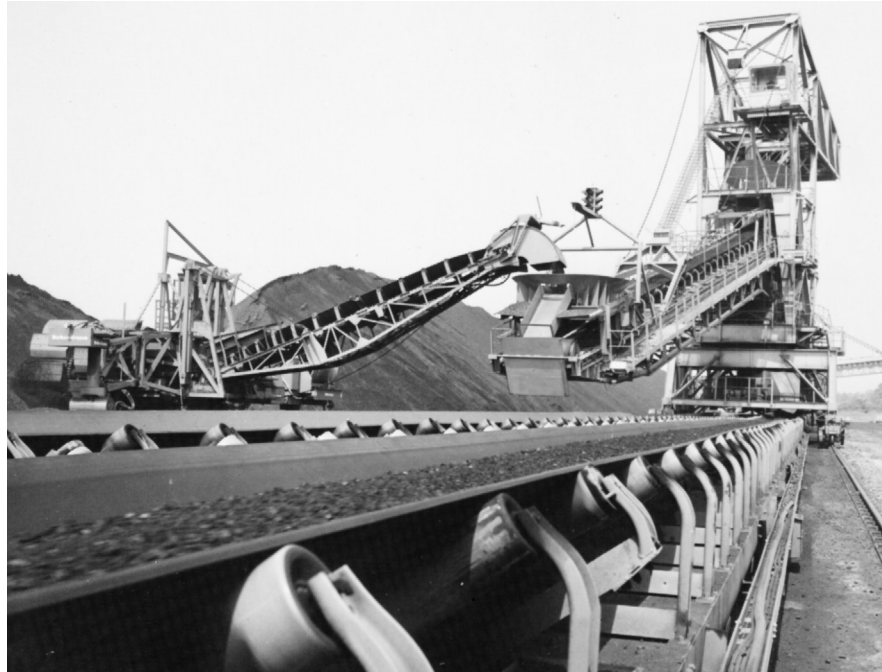
Figure 2.23 Crawler-mounted bucket wheel reclaimer with wheel mounted on chassis discharges onto a rail-mounted reclaim conveyor with slewing boom.
