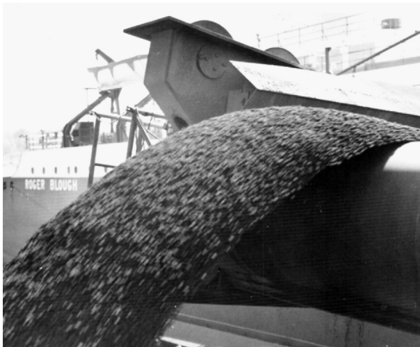
Figure 12.53 Iron-ore pellets discharging from boom belt of Great Lakes self-unloader ship at 10,000 tph.
