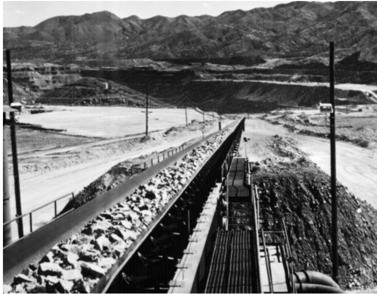
Figure 1.1 60-inch conveyor carries large lumps of abrasive ore on incline.
