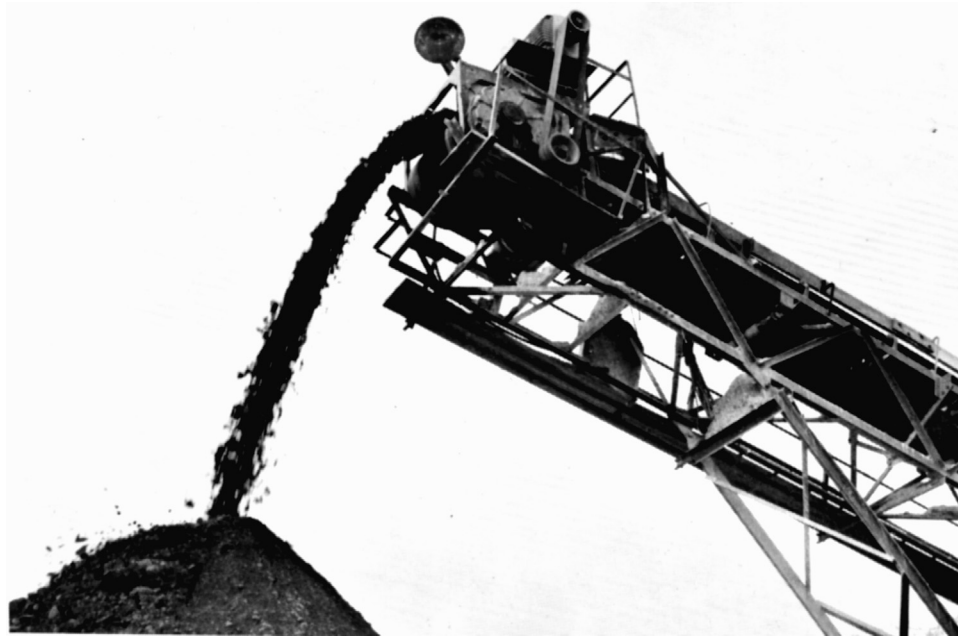
Figure 12.52 Sized aggregate pours over end pulley of this inclined conveyor.
