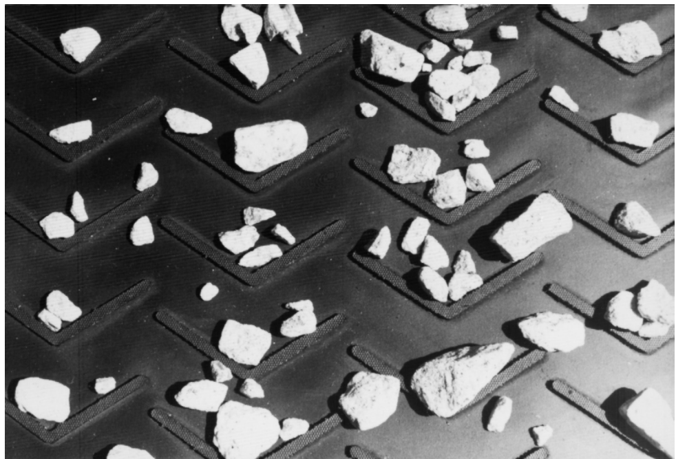
Figure 10.1 Example of molded chevron cleated belt.
