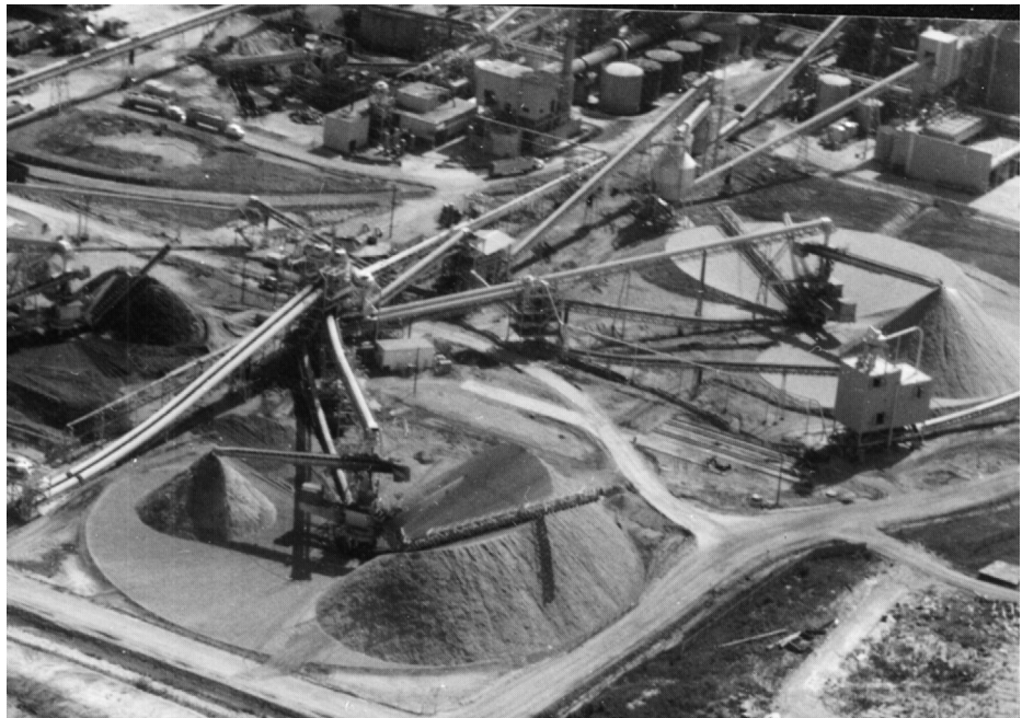
Figure 1.12 Circular stacker reclaimer simultaneously stacks and reclaims over 3,000,000 cubic feet of wood chips at a major paper mill.
