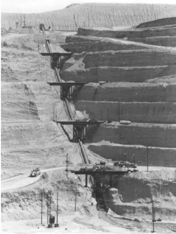
Figure 1.6 Multiple loading stations feed ore to slope conveyor in open-pit mine.
