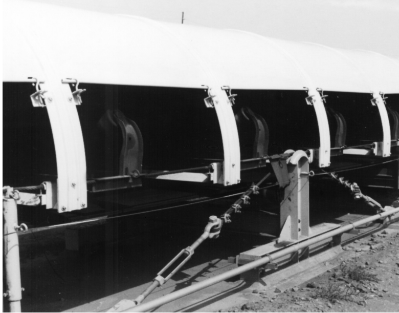
Figure 1.4 Corrugated metal cover over the belt provides weather and environmental protection.
