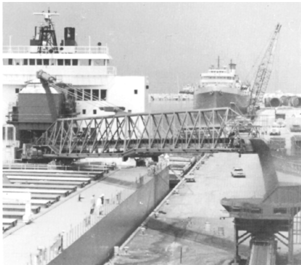
Figure 1.14 Self-unloading ship with 78-inch discharge conveyor unloads iron ore pellets at 10,000 tph.
