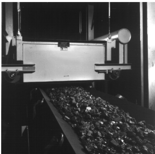
Figure 1.16 V-type plow diverts foundry sand from flat belt conveyor.
