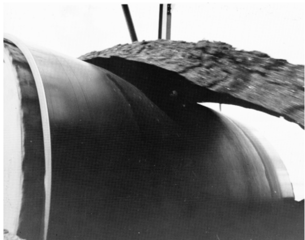
Figure 12.54 Close-up of trajectory from head pulley of conveyor, speed 760 fpm, handling iron-ore pellets.
