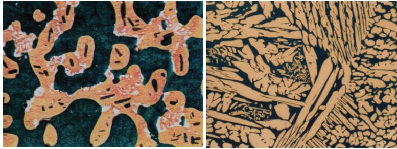
Fig. (23). The microstructure of F-A cast steel in the as-cast conditions (a-Magn.800X – white areas are carbides) and after solution annealing (b- Magn.400X – yellow areas – austenite, dark - ferrite).
