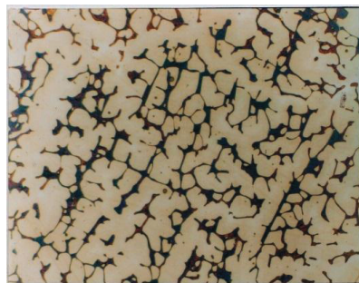
Fig. (10). The microstructure of cast duplex steels with different nitrogen contents [16].
