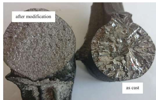
Fig. (9). Effect of modification by Fe – Ti on the primary grain size [19].
