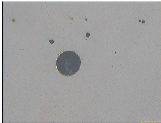
Fig. (14). Macro-inclusion (silicate) in carbon cast steel, Magn.250X.
