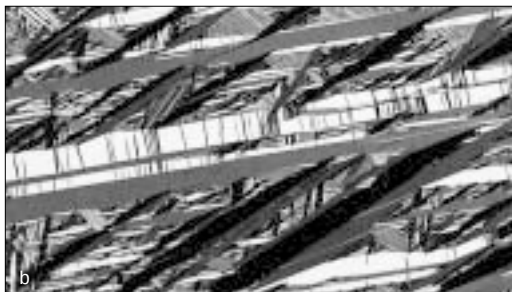
Figure 46. Martensitic microstructure of heat treated, eutectoid aluminum bronze (Cu-11.8% Al) in the unetched condition viewed using: a) bright field illumination, b) polarized light
