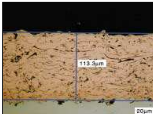
Figure 56. An example of an operator estimating coating thickness with the use of a parallel tool.
