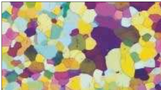
Figure 38. Grain structure of annealed CP titanium revealed by heat tinting on a hot plate (100X, polarized light plus sensitive tint).
