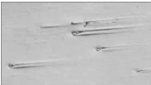
Figure 21. "Comet tails" at large nitrides in an annealed H13 hot work die steel specimen (200X, DIC).
