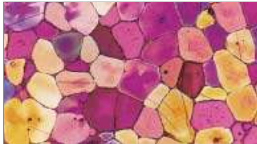
As-cast microstructure of a magnesium alloy with 2.5% of rare earth elements, 2.11% Zn and 0.64% Zr showing a film of the rare earth elements in the grain boundaries, alloy segregation within grains ("coring" revealed by color variations within grains) and a few mechanical twins in the grains (acetic-picral etch, crossed polarized light plus sensitive tint, 100X).
