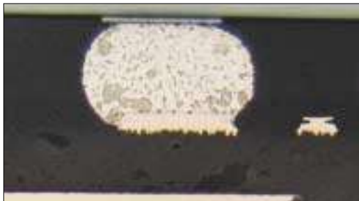
Silicon flip chip, solder balls, on PC board, (200x).
