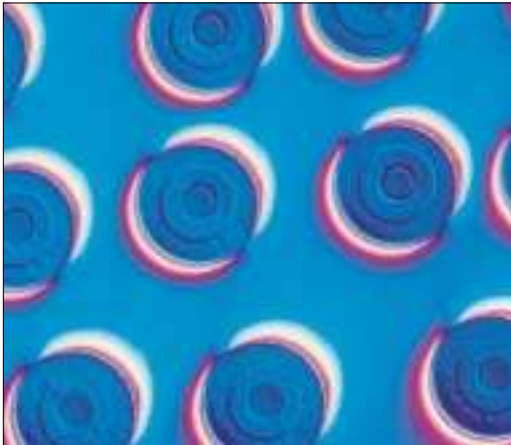
Microstructure of a metal-matrix composite, SiC in a CP titanium matrix (unetched, Nomarski DIC, 100X).
