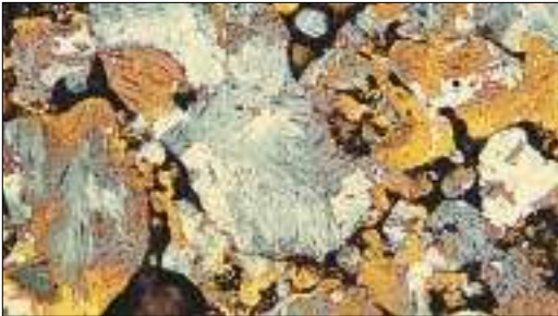
Lath martensitic microstructure of an unconsolidated powder metallurgy steel gear containing substantial porosity (Klemm's I reagent, polarized light, 200X).
