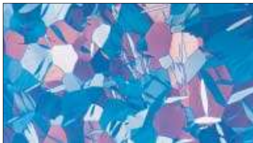
Figure 30. Mechanical twins at the surface of hot worked and cold drawn high-purity zirconium viewed with polarized light (200X).
