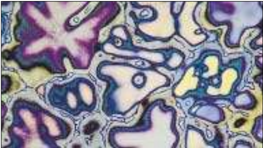
Dendritic segregation in as cast 206 aluminum revealed by color etching with Weck's reagent (polarized light, 200X).
