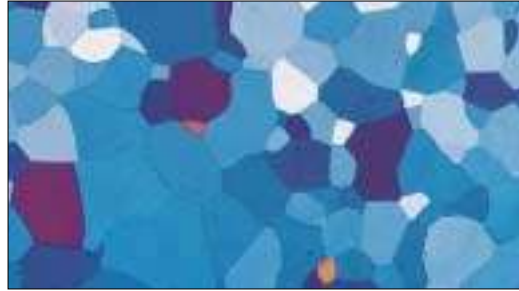
Equiaxed grain structure of wrought hafnium (unetched, crossed polarized light plus sensitive tint, 100X).
