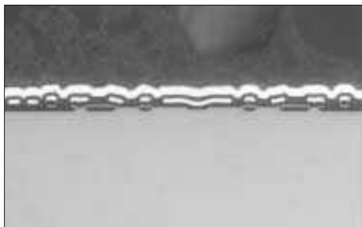
Aluminum circuitry on silicon adjacent to mineral filled epoxy packaging, (1000x).
