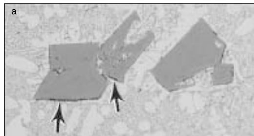
Figure 23. Examples of freedom from relief (a, top) and minor relief (b, bottom) at the edges of large primary hypereutectic silicon particles in an as-cast Al-19.85% Si specimen (200X, aqueous 0.5% HF).
