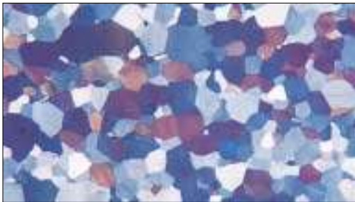
Equiaxed grain structure of wrought zirconium (unetched, crossed polarized light, 100X.)
