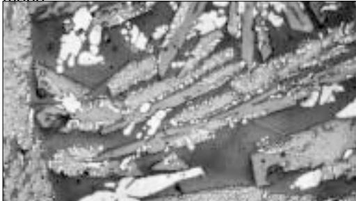
Microstructure of an alumina (matrix), zirconia (gray), silica (white) refractory material (unetched, 200X).
