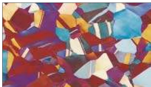
Alpha grains containing annealing twins in phosphorous-deoxidized arsenical bronze that was annealed and lightly cold drawn (Klemm's I reagent, polarized light, 50X).
