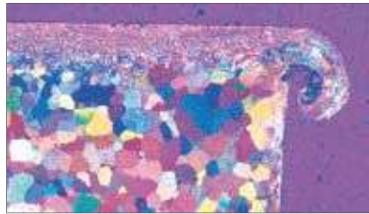
Figure 2. Cutting damage (top) and a "burr" after sectioning of an annealed CP titanium specimen (mod. Weck's reagent, 100X, polarized light plus sensitive tint).
