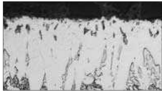
Figure 6. Excellent edge retention of a borided 42CrMo4 alloy steel specimen mounted in Epomet resin (1000X, 2% nital).
