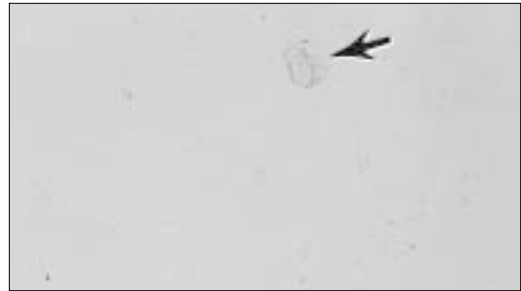
Figure 22. Staining (arrow) on the surface of a of Ti-6% Al-2% Sn-4% Zr-2% Mo prepared specimen (200X).
