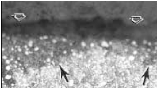
Figure 10. Staining (thin arrows) due to etchant bleed out from a shrinkage gap (wide arrows) between the phenolic mount and the M2 high speed steel specimen (500X, Vilella's reagent).
