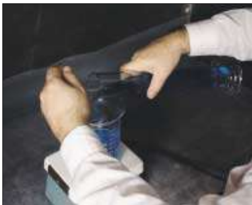
Figure 64. When mixing etchants, use a magnetic stirring plate with a magnetic bar for stirring. Slowly add the liquid ingredients to the solvent by dripping them down a glass stirring rod. If the solution is more dangerous than this one, wear protective gloves and use a face shield. If mixing generates substantial heat, it is a good practice to place a cooling jacket around the beaker.
