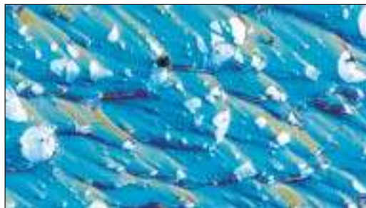
Micrograph of high-density polyethylene containing a filler (white particles) (unetched, Nomarski DIC, 100X).
