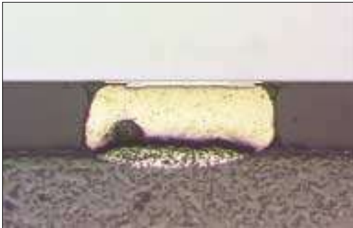
High temperature (96% Pb) solder under flip chip on ceramic substrate, (200x).
