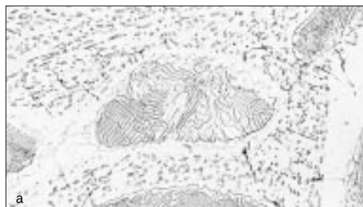
Figure 32a. The ternary eutectic ( \alpha - \text{Fe}_3\text{C} - \text{Fe}_3\text{P} ) in gray cast iron revealed by etching (a, top) in picral and nital to "outline" the phases
