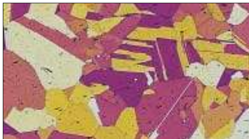
Alpha grains containing annealing twins of solution annealed and double aged Waspalloy nickel-based superalloy (Beraha's reagent, 100X).
