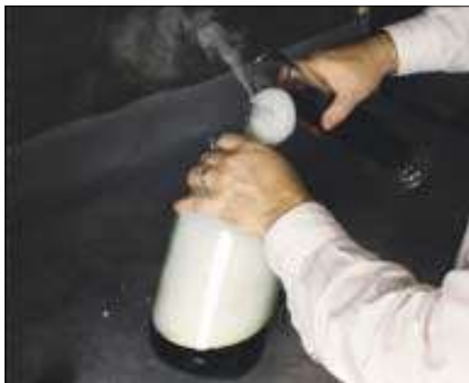
Figure 65. Illustration of a bad mixing practice. The acid ingredient was poured into an empty acid bottle and the solvents were added without stirring or cooling. The solution may erupt in the metallographer's face at any moment. It is recommended to keep the hands clear of the area and remove rings.
