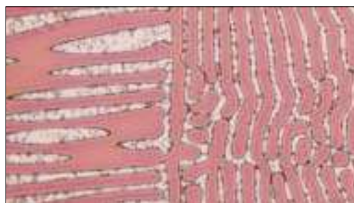
Figure 35. Theta phase, CuAl_2 , colored in the \alpha -Al - \epsilon eutectic in an as-cast Al-33% Cu specimen by immersion color etching with the Lienard and Pacque etch (200 mL water, 1 g ammonium molybdate, 6 g ammonium chloride) at 1000X.
