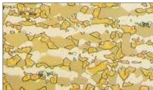
Microstructure of a duplex (ferrite tan, austenite white) stainless steel held at 816° C for 48 hours which forms sigma phase (orange particles) revealed by electrolytic etching with aqueous 20% NaOH at 3 V dc, 9 s (500X).
