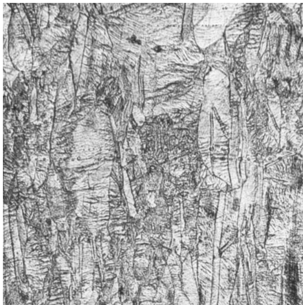
Figure 4.3 Corrosion of brass cold-worked 60%. Magnification 150X.
