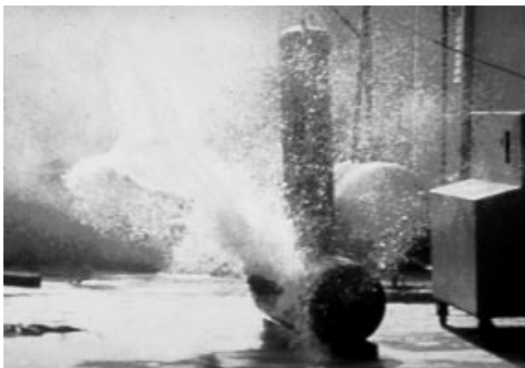
Figure 1.6 Primary stress failure.
