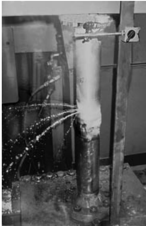
Figure 1.8 Secondary stress (fatigue) failure crack.
