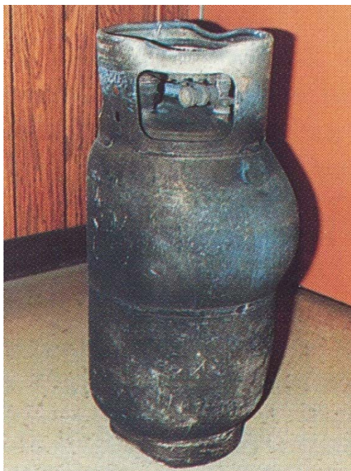
Figure 6—Fire damaged cylinder exhibiting bulging
