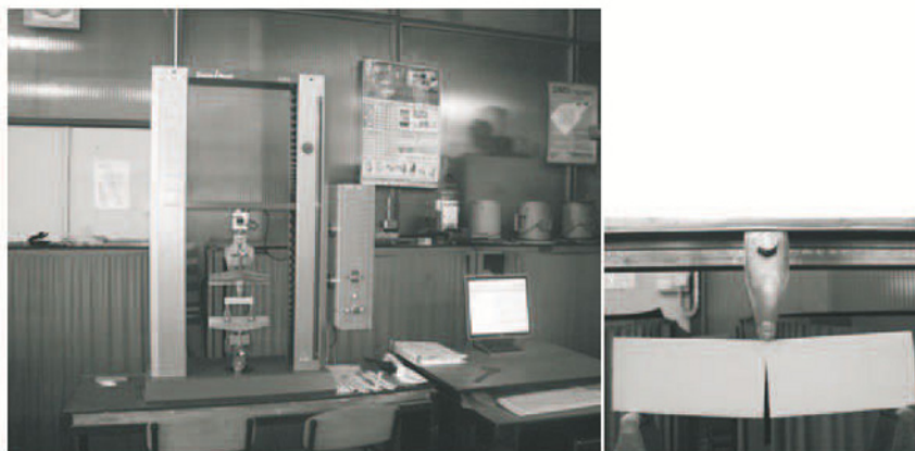
Figure 17. Testing machine and detail of a fractured specimen during test: Zwick/Roell testing machine (left), detail of fractured specimen (right)
