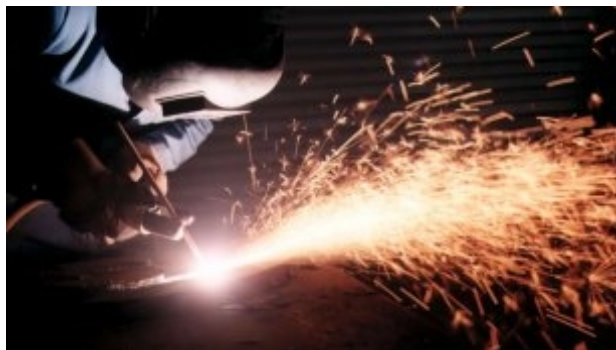
Figure 18.3 Thermal excavation using arc/air gouging.
