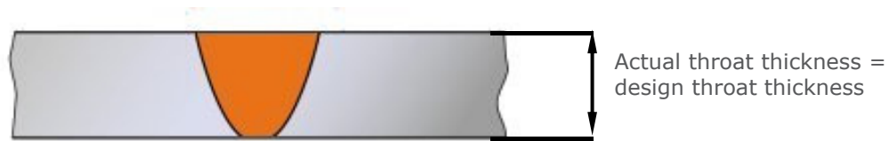
Figure 2.22 Full penetration butt weld ground flush.
