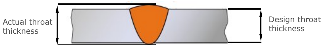
Figure 2.20 Full penetration butt weld.
