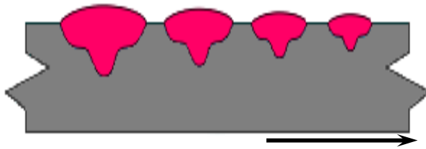
Figure 13.8 The effect of travel speed. As travel speed increases, reducing penetration and width, undercut.
