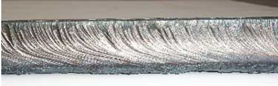
Figure 15.4 Effect of excessive travel speed.
