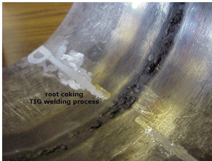
Figure 3.31 Temper colour of stainless steel.
