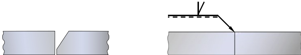
Figure 9.5 Single bevel butt joint representation.
