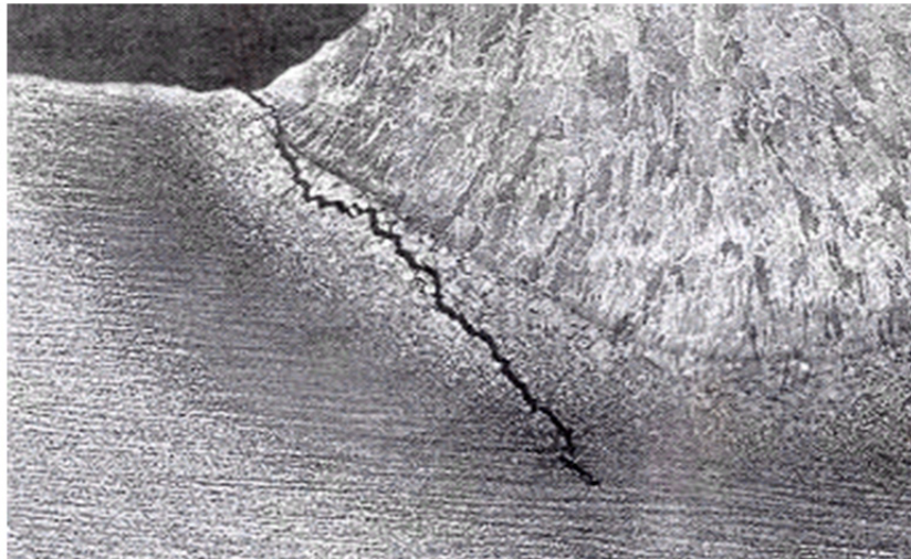
Figure 17.2 Hydrogen induced cold crack that initiated at the HAZ at the toe of a fillet weld.
