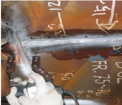
Figure 5.8 Magnetic particle inspection using a yoke.
