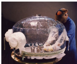
Welding in protective tent
