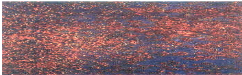
Figure 7.4 Rust Grade B.
