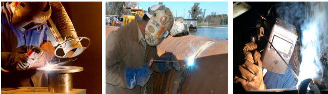
Figure 11.2 Examples of the MMA welding process.
