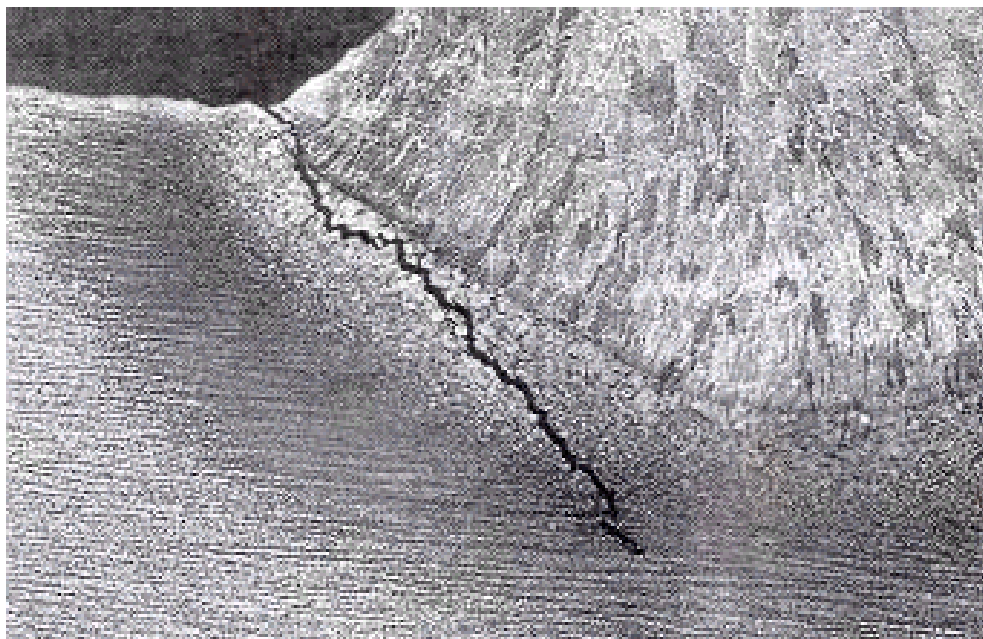
Figure 11.2 Hydrogen induced cold crack that initiated the HAZ at the toe of a fillet weld.
