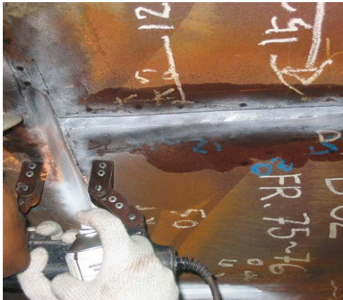
Figure 14.8 Magnetic particle inspection using a yoke.
