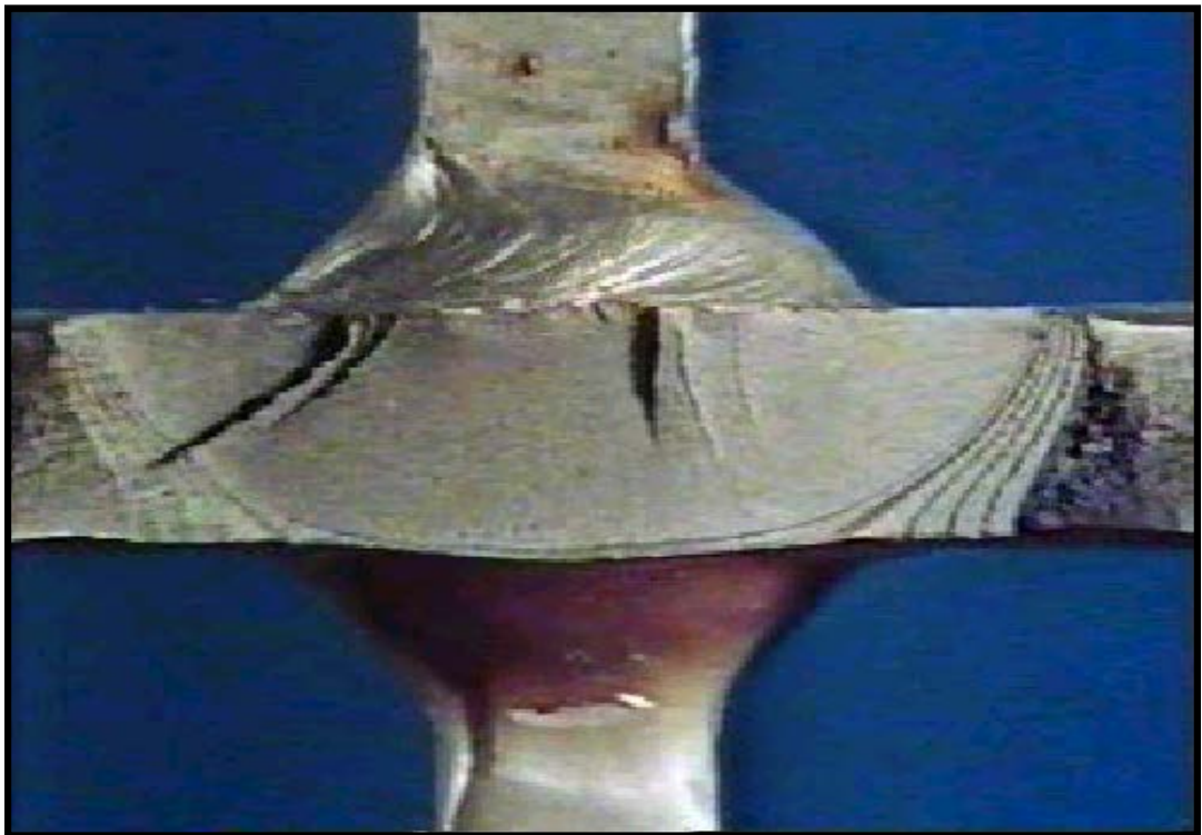
Typical fatigue fracture in a T joint.
