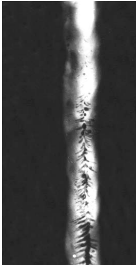
Figure 14.3 X ray of a welded seam showing porosity.
