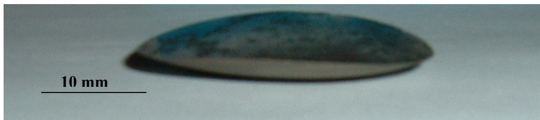
Figure B2.3 (a) An electro-discharge machining sample removal system [13] and (b) example of a sample removed with the system.
