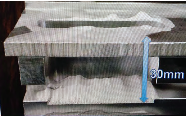
Fig. 9.22 Slot in Al-7075 missile rail in the as-sprayed condition. Courtesy of South Dakota School of Mines and Technology
