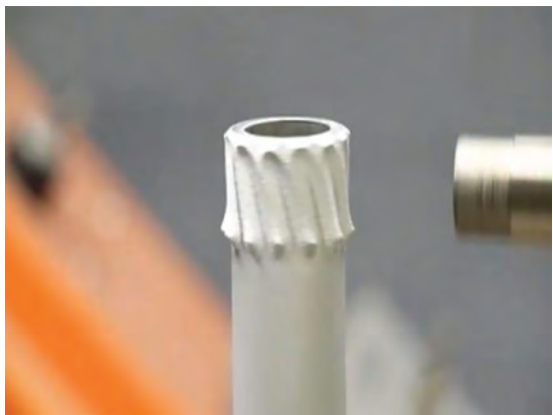
Fig. 8.3 Practical example of shaft fabrication via cold gas dynamic spraying additive manufacturing technology, which was conducted by General Electric. Source: Ref 8.28
