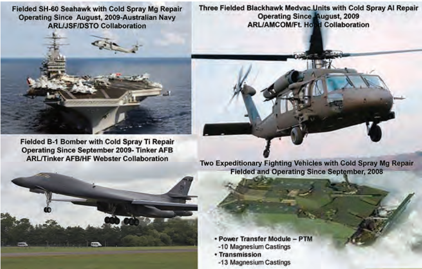
Fig. 11.14 Cold spray repair applications, from prototype to the field. Source: Ref 11.2
