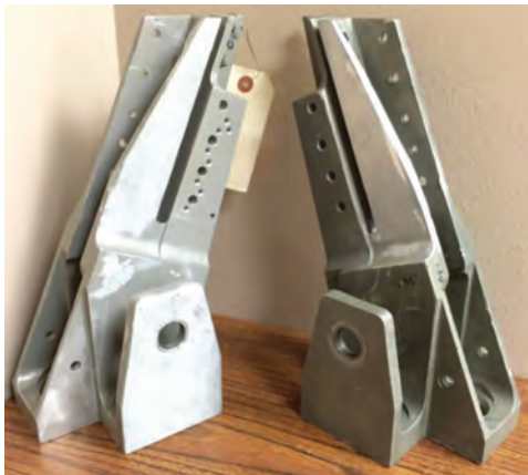
Fig. 9.24 Hinge fittings made from Al-7075-T6 that can be repaired without being removed from the aircraft. Courtesy of South Dakota School of Mines and Technology
