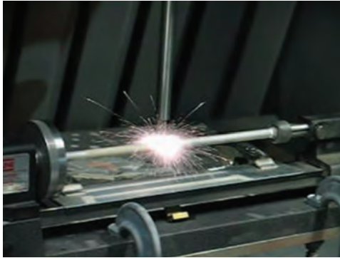
Fig. 9.26 Application of commercially pure titanium on 9.5 mm (0.4 in.) Haynes AMS 4944 (Ti-3Al-2.5V) hydraulic tubing. Courtesy of South Dakota School of Mines and Technology
