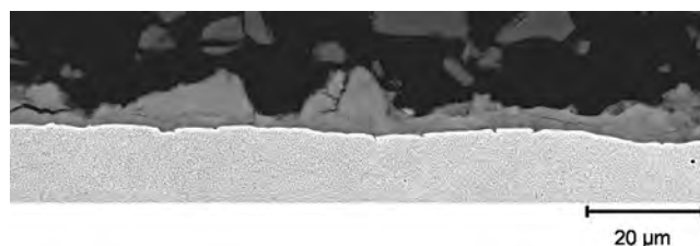
Fig. 2.11 SEM cross-sectional micrograph of a cold-sprayed TiO 2 coating on a stainless steel substrate that consists of multiple layers of primary particles. The ceramic layer shows some cracks. Source: Ref 2.67
