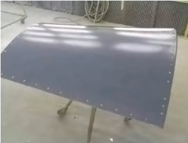
Fig. 9.11 Fully repaired forward equipment bay panel ready to be put back into service. Courtesy of South Dakota School of Mines and Technology
