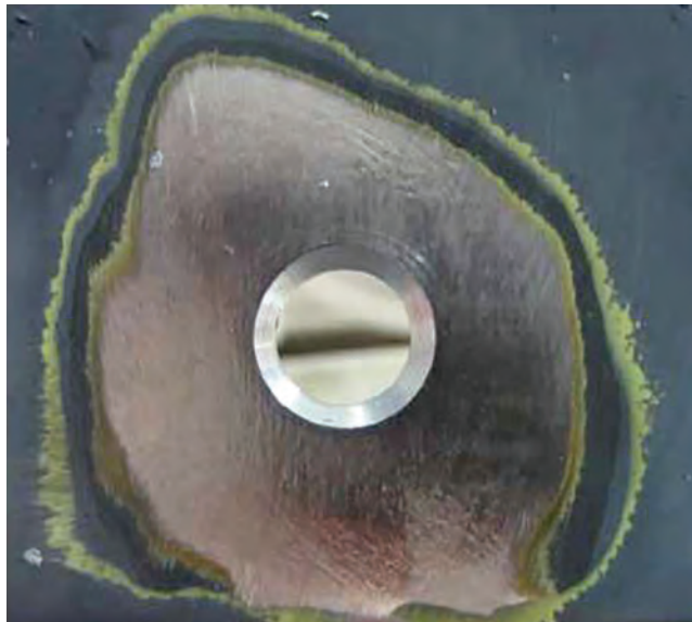
Fig. 9.10 High-pressure cold-spray-repaired and machined fastener hole in a forward equipment bay panel. Courtesy of South Dakota School of Mines and Technology
