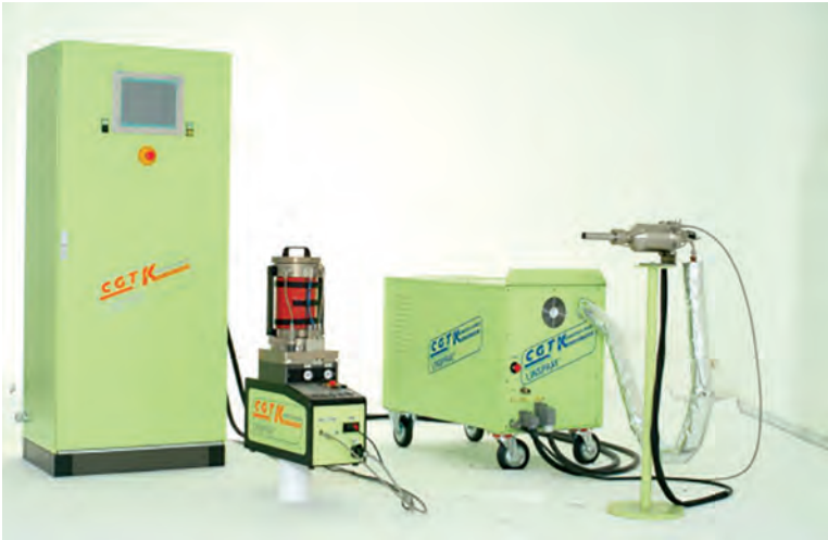
Fig. 4.2 KINETIKS 4000-47 (30 kW preheater) system
