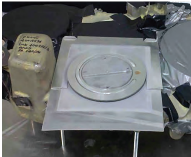
Fig. 9.4 Hydraulic mounting pad on the A357 transmission housing. Courtesy of the Applied Research Laboratory, The Pennsylvania State University
