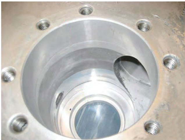
Fig. 9.17 Final machining performed on the repaired actuator. Courtesy of Puget Sound Naval Ship Yard
