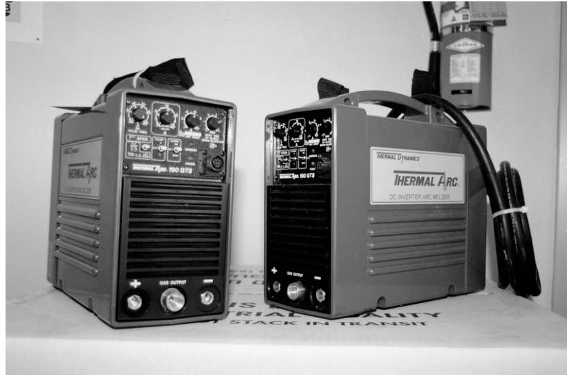
Figure 4.5: Portable inverter type constant current power source.
