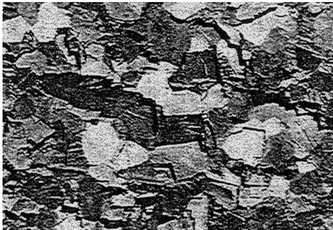
Figure 7.5: Surface of brittle fracture. The shiny facets result from the cleavage of the individual grains giving a crystalline appearance.
