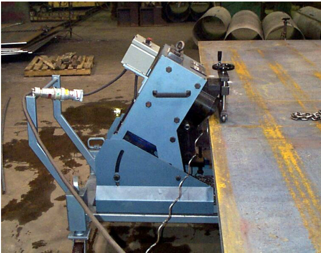
Figure 3.24(a): Rotary shear. (Photo courtesy of Gullco International)
