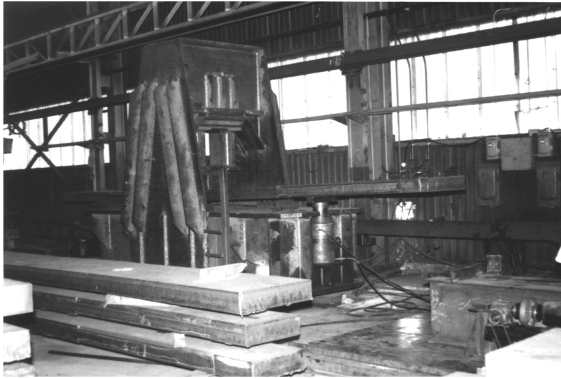
Figure 6.49: Specially designed straightener. (Courtesy of Canon Inc.)
