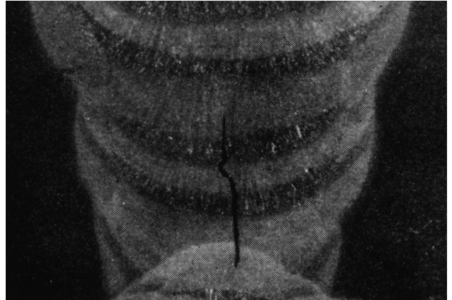
Figure 9.57: Root crack in thick U butt.
