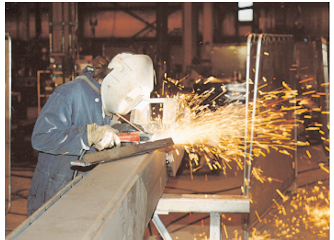
Figure 3.22(b): Principle of air carbon arc process.
