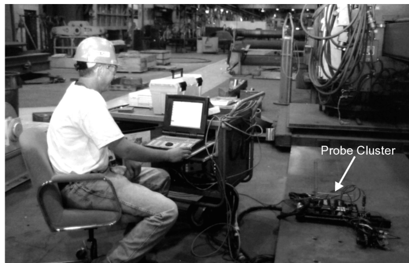
Figure 9.94: Fully automatic ultrasonic testing machine. (Photo Courtesy of Babcock & Wilcox Canada)
