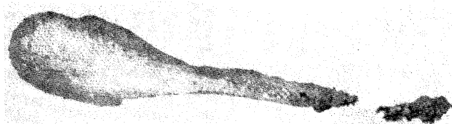
Fig. 5-5. Close-up of shrinkage from gassy C95400 alloy poured in a 1-in. chilled Y-block. In this case the cavity is smooth.
