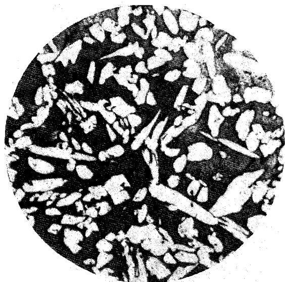
Fig. 10-1. As-cast (sand) microstructure of alloy C86500 (58% Cu, 0.5% Sn, 39.5% Zn, 1% Fe, 1% Al). Light, acicular alpha phase in beta matrix. (100x)
