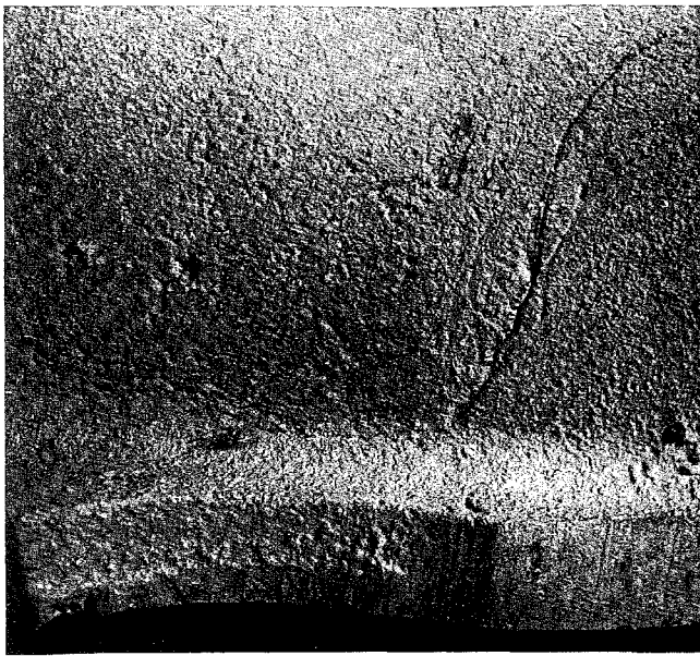
Fig. 15-29. Casting with oxide film inclusions. The metal entered the mold with turbulence, and aluminum oxide skins were trapped in the casting wall.
