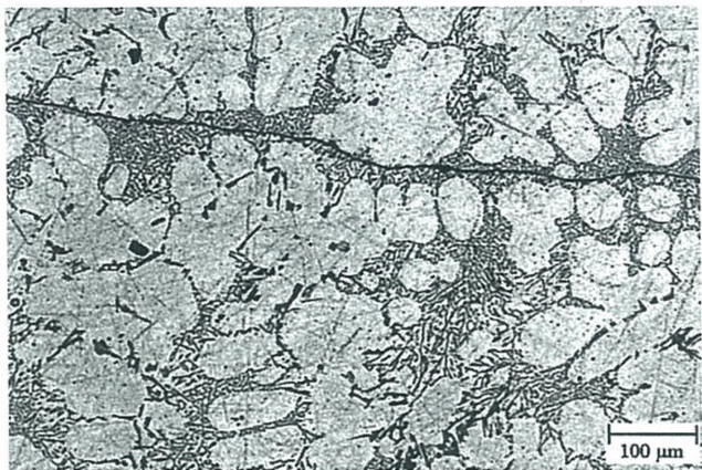
Fig. LF-6. Photomicrograph of fold defect in 356, located in interdendritic region of the eutectic, last area to solidify.
