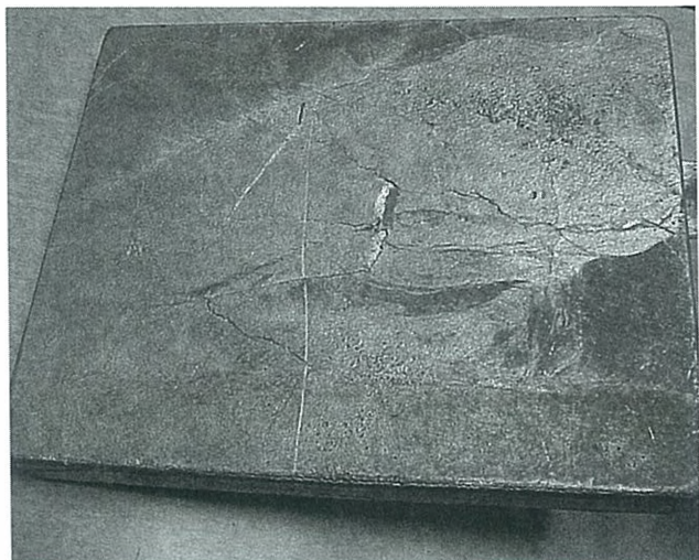
Fig. SC-5. Buckles on a plate casting.
