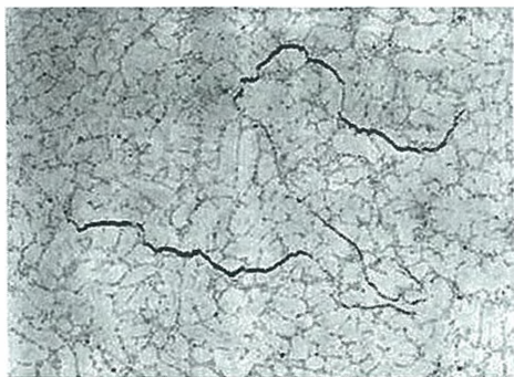
Fig. PM-60. Microstructure showing inter-granular new (from pouring) and old (melting and/or prolonged holding) oxide skins.
