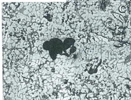
Fig. SC-45. Undissolved Al-Sr-Si from modifier addition.
