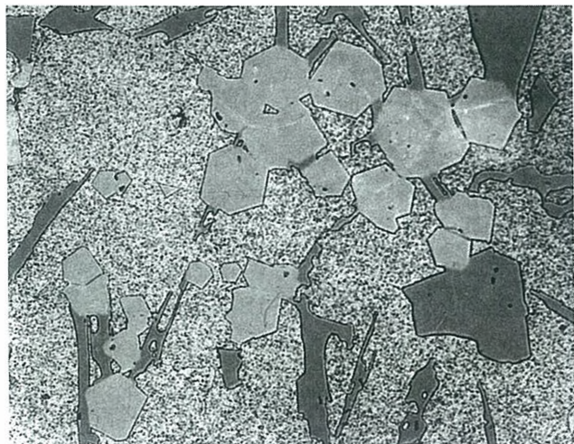
Fig. DCM-6. Microstructure of "metallurgical sludge"—polyhedral shape.
