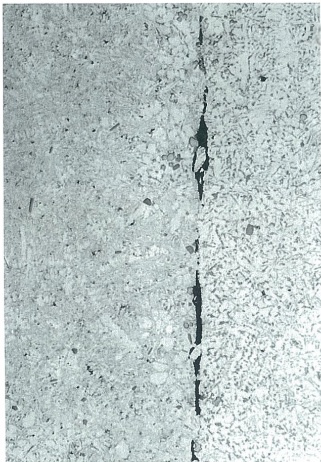
Fig. DCP-5. Cold lap, knit line.
