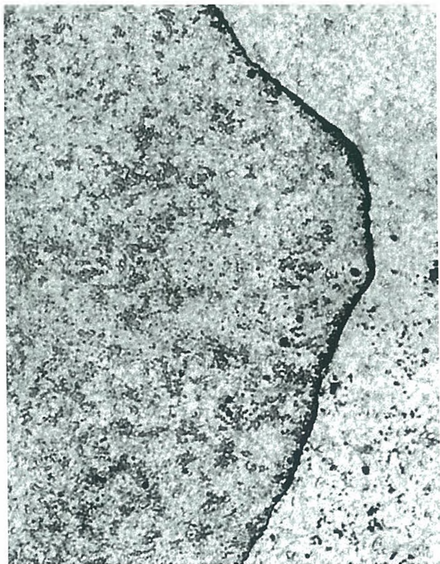
Fig. DCP-6. Severe cold shut and /or lap on 380 alloy.
