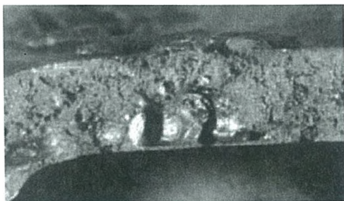
Fig. SC-42. Oxides found in fracture site on a casting.
