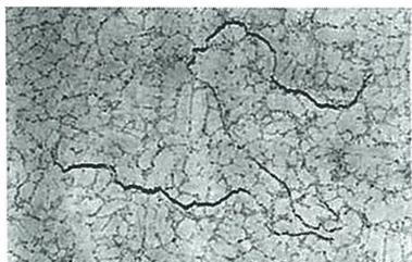
Fig. PM-33. Photomicrograph of hot tear along grain boundary.
