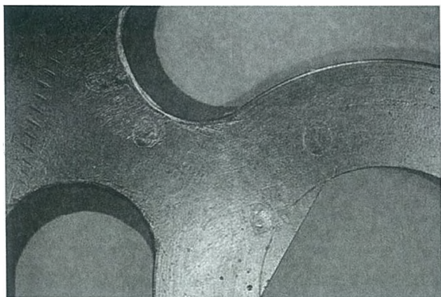
Fig, IC-19. Cold shut.
