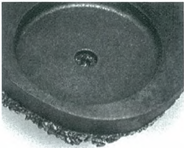
Fig, IC-12. Shell cracking; flashing.
