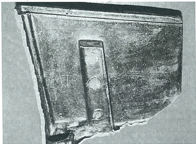
Fig. PC 3. Metal-mold reaction due to residual moisture in the plaster.
