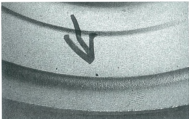
Fig. SC-49. A356 inclusion from shell core breakdown or dross entrained in pouring.
