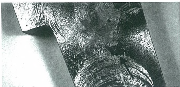
Fig. SC-46. Hard spot (oxide or intermetallic) in 319 casting.
