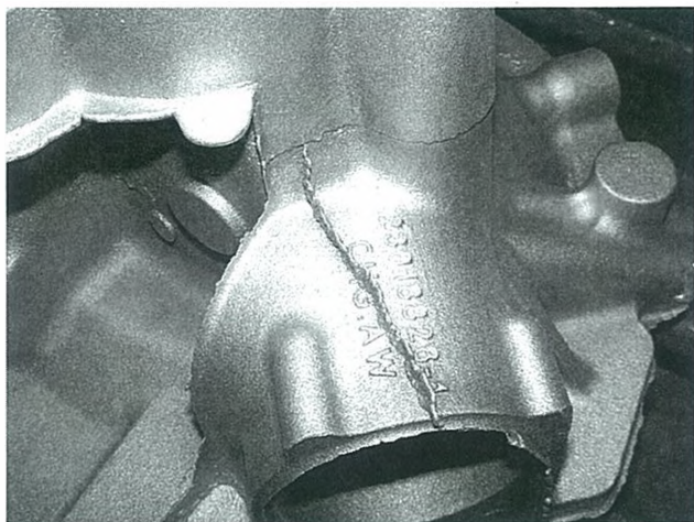
Fig. SC-1. Mold crack.
