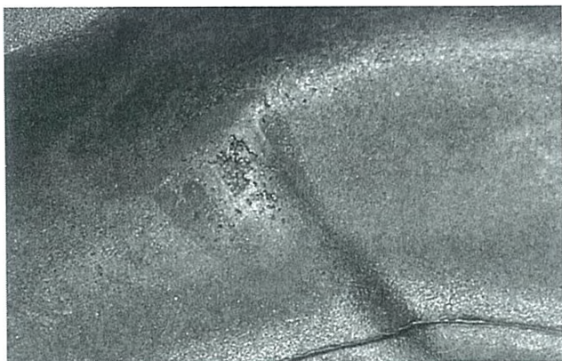
Fig. PM-49. Surface shrink due to insufficient metal volume or low pour temperature.
