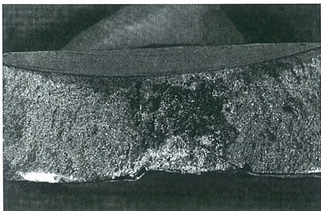
Fig. SC-18. Internal sponge observed with zygo (black light) caused by inadequate feeding and/or poor solidification.
