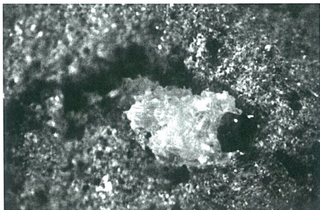
Fig. DCM-10. Flux inclusion.
