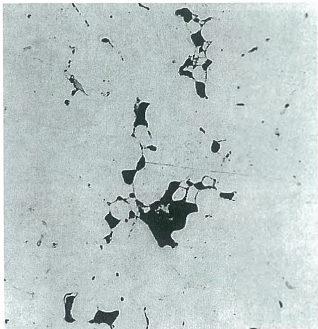
Fig. PM-53. Gross micro shrinkage.
