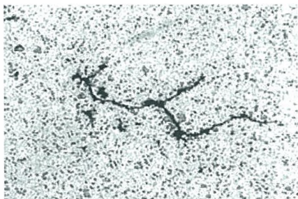
Fig. DCM-8. Oxides in 380 alloy.
