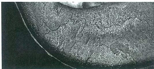
Fig. PM-2. Rough surface from excessive die coating application.
