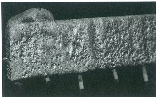
Fig. LF-28. Surface undulations on the casting resulting from entrapment of liquid-EPS at the metal-coating-mold interface.
