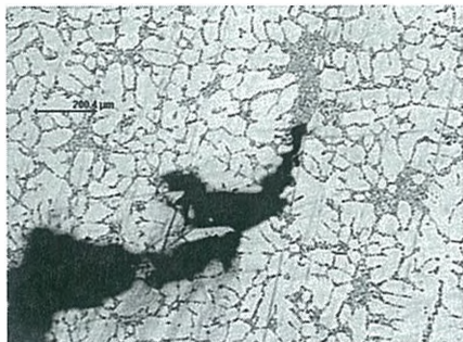
Fig. SC-25. Hot microtear.
