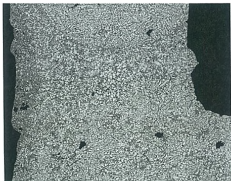
Fig. LF-17. Microstructural segregation at a glue joint in A356 aluminum.
