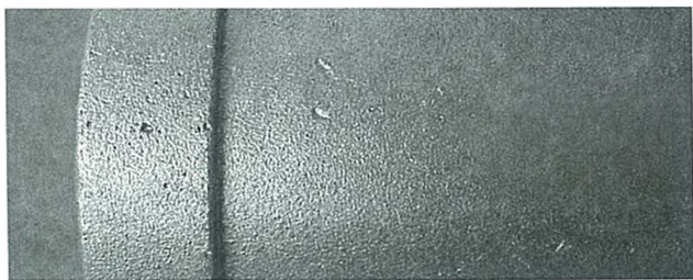
Fig. SC-48. A356 alloy; dross or inclusion on cope surface near ingate; remedied by adjusting pouring practice.
