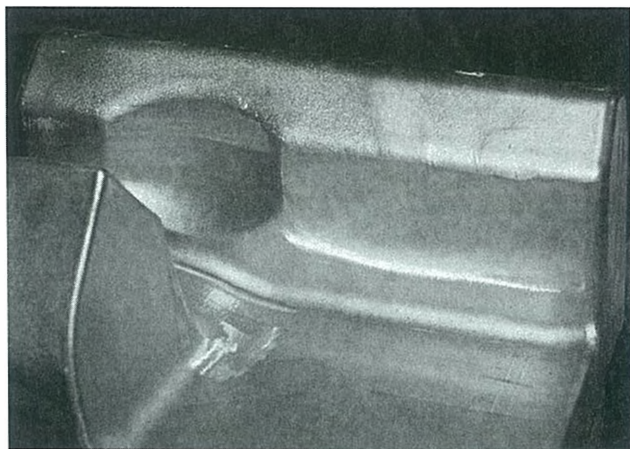
Fig. PM-47. Shrinkage due to insufficient riser volume.
