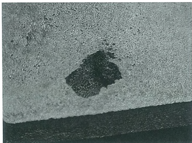
Fig. SC-7. Erosion near gating on 356 alloy casting.
