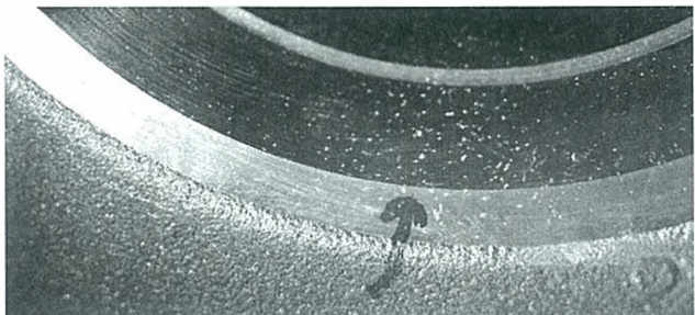
Fig. PM-34. Dispersed surface and/or sub-surface porosity caused by hydrogen.
