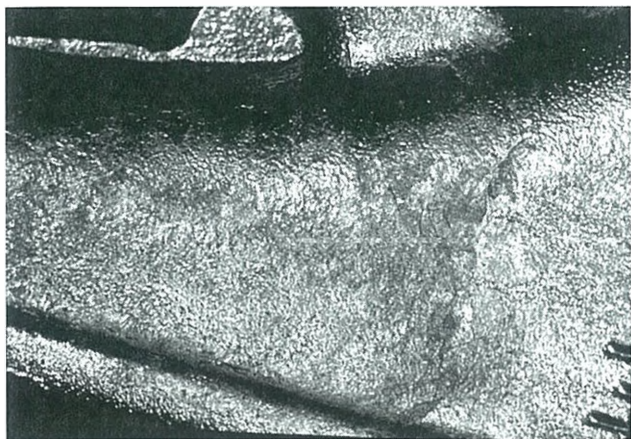
Fig. SC-39. Oxide films folded into casting during solidification.
