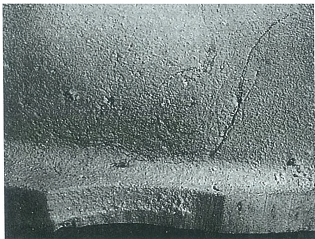
Fig. SC-38. Oxide film inclusion in green sand casting due to turbulence during filling.
