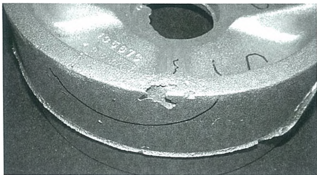
Fig. SC-9. Hole on casting surface caused by loose sand.
