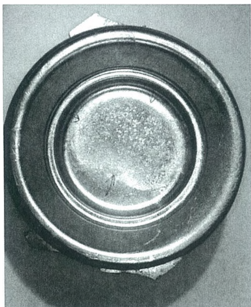
Fig. PM-45. Shrinkage in center due to poor casting design (heavy outer band).
