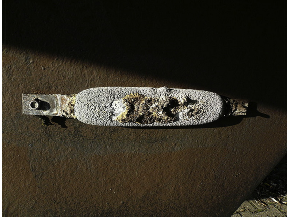
Figure 1.1 Galvanic sacrificial anode attached to the hull of a ship.
