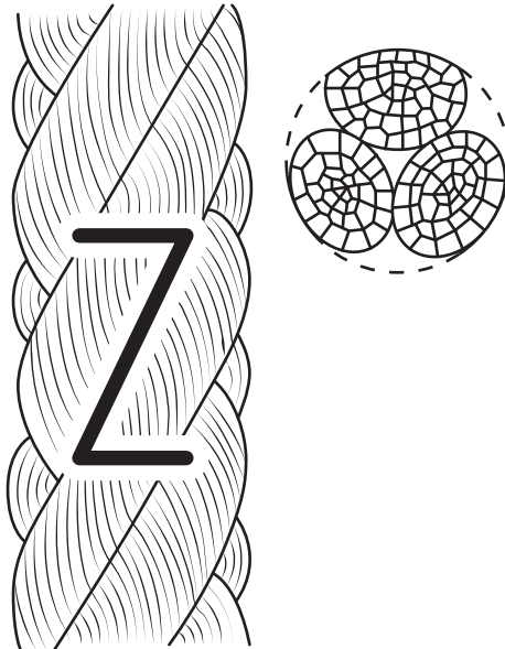
Figure 4.9 Three-strand (plain or hawser laid) “Z” or right-hand lay rope.
