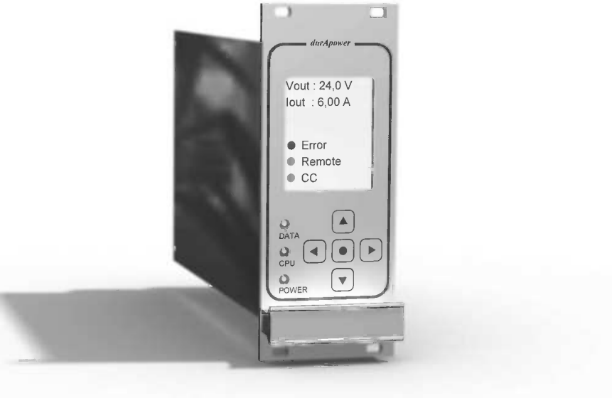
Figure 10.7 Switch mode board and display.
