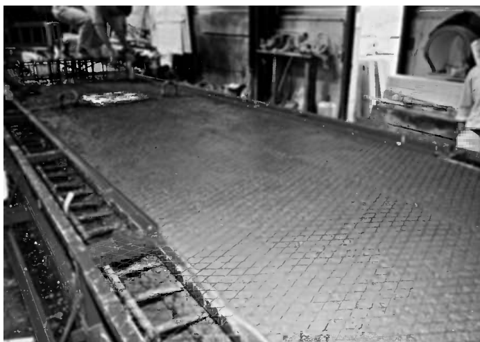
Figure 9.3 CP anode integrated within precast deck slab.
