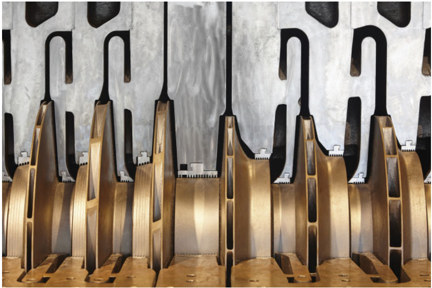
Figure 8.1 A cutaway of a centrifugal compressor showing the rotor and diffusers.
