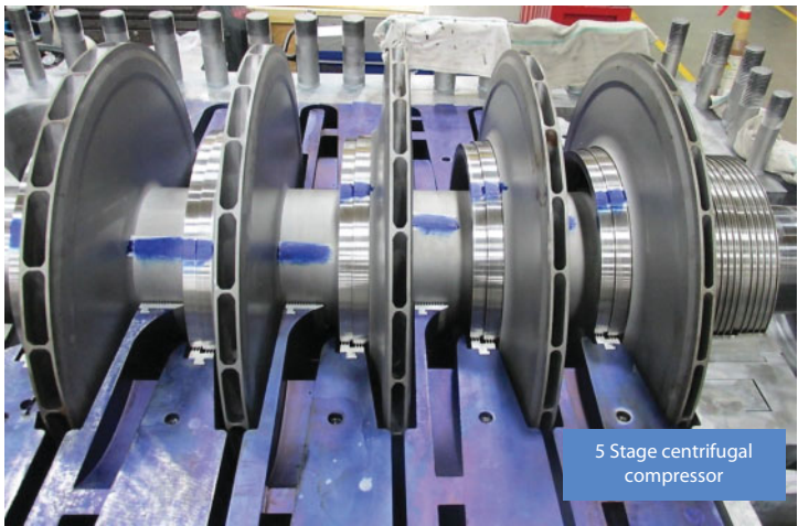
Figure 6.2 Compressor rotor inside of a split casing. Notice that every impeller exit vanes line up with a corresponding diaphragm.
