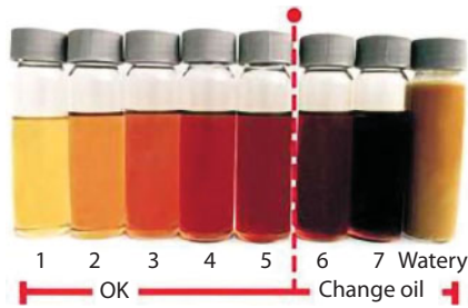
Figure 17.5 How oil appearance can change as it becomes contaminated. Remember to look for changes from newly installed oil.
