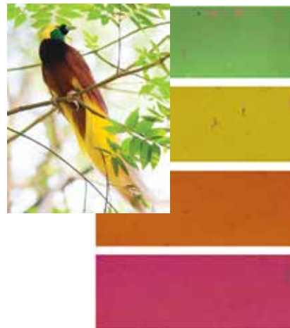
▲ Chemists produced nanoparticles of synthetic melanin and dried them into thin films to create a range of pure hues. The arrangement of the particles, rather than different kinds of pigments, determines the colors. Image courtesy of UCSD and the Univ. of Akron.
