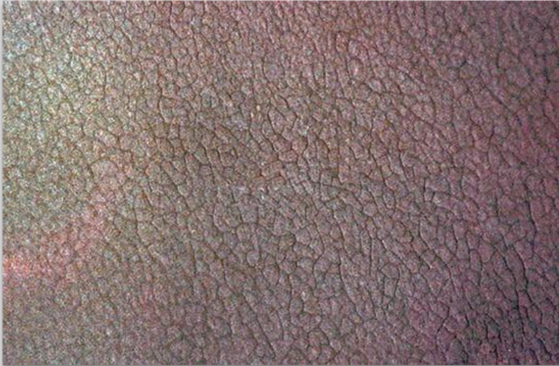
Fig. 25 The dried paint film has the appearance of a dried-out mud flat. The cracks appear as a network that can vary in size and amount.
