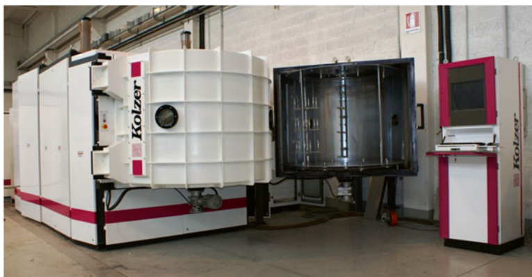
Fig. 13.5 Two-door batch vacuum metallizer (KOLZER)
