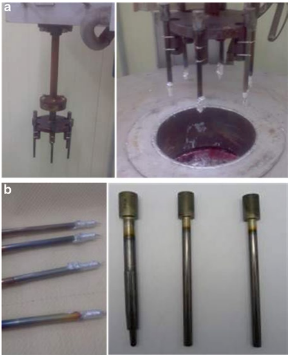
Fig. 9.10 Dipping and rotating test in Al bath for comparison of adhesion behavior. (a) Coated pins dipped into Al bath before ( left ) and after ( right ). (b) Al stuck pins ( left ), after NaOH washed pins ( right )
