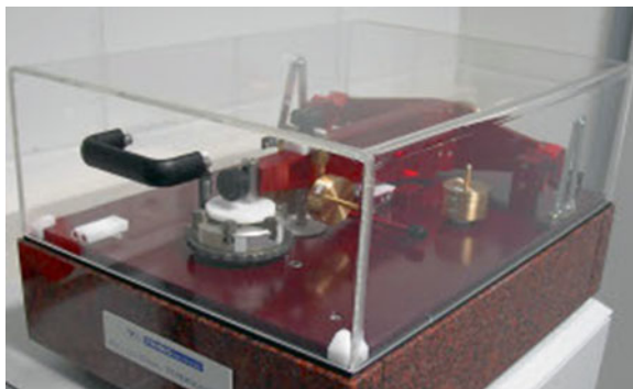
Fig. 7.2 Oscillating ball-on-disk tester (Source: Photo IHI Ionbond)
