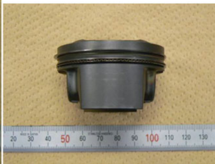
A2618⇒DLC coating applied after W shot-peening and light polishing Cylinder bore : PCVD DLC
