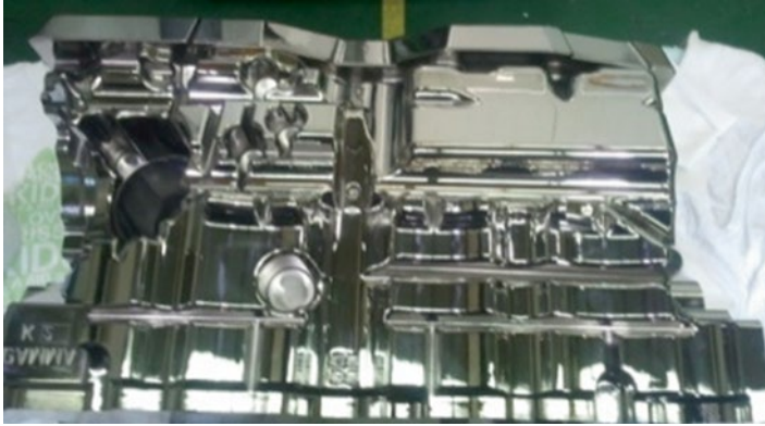
Fig. 9.16 TiAlCrSiCN-coated Gamma engine block No. 3 die
