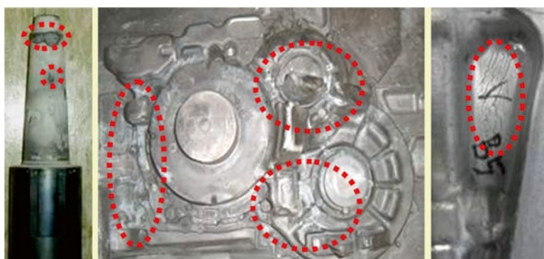
Fig. 9.4 Damages on die surfaces – Al stuck, surface cracked
