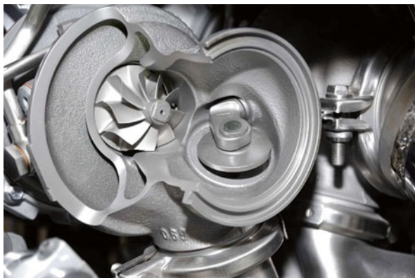
Fig. 7.6 View of the turbine section of a generic turbocharger. Wastegate and turbine impeller are shown (Source: Fotolia LLC, www.fotolia.com )
