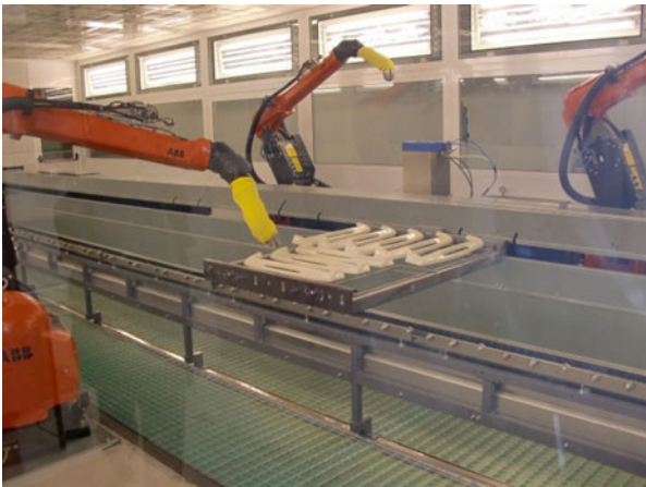
Fig. 13.14 Robot painting on horizontal frames
