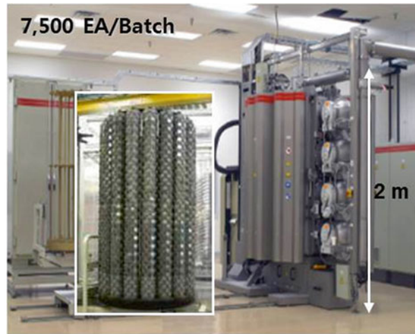
Fig. 2.1 PVD machine for DLC-coated tappets
