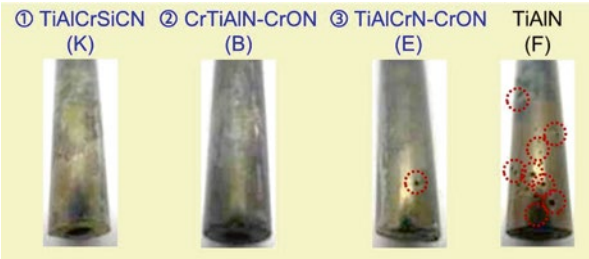
Fig. 9.13 Images after adhesion test—excellent coatings (K, B, E ranked) after 27 h, TiAlN after 6 h, adhesion test
