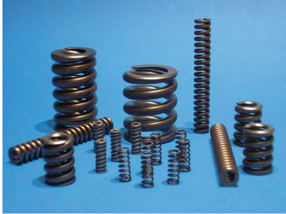
Fig. 6.12 Springs treated by the low-temperature GN process (METANIT) (courtesy of Oerlikon Metaplas)
