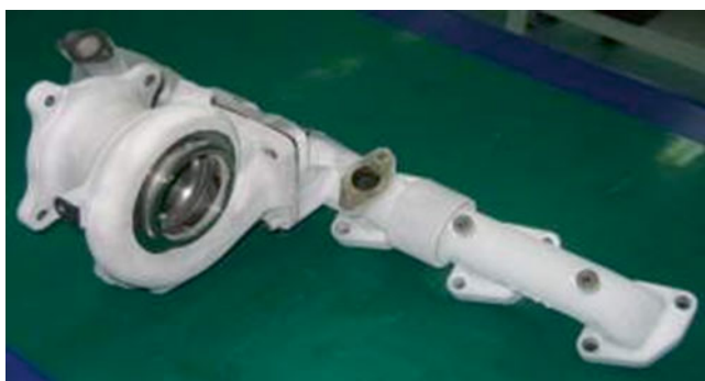
Fig. 2.11 YSZ sprayed exhaust parts
