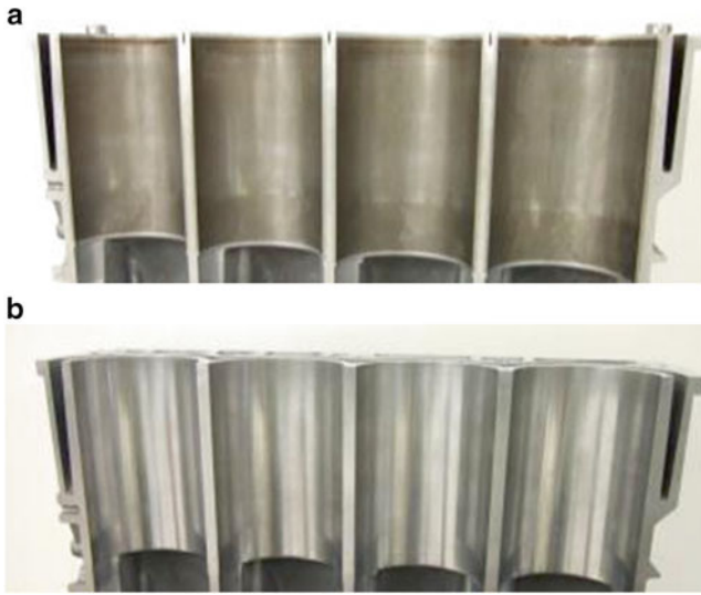
Fig. 4.13 Photograph of an engine block cross section showing (a) cast iron and (b) PTWA surface following honing
