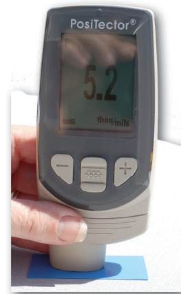
Place gage probe on high shim
