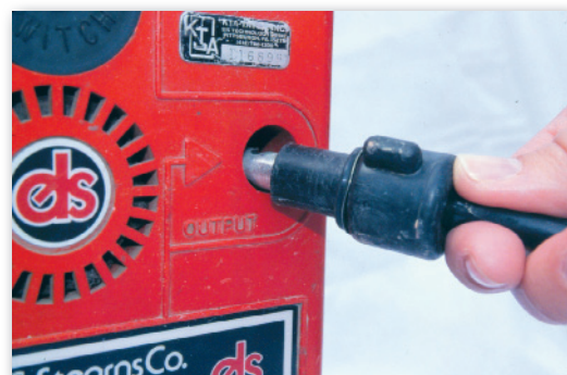
Insert electrode cable connector into detector port “OUTPUT”
