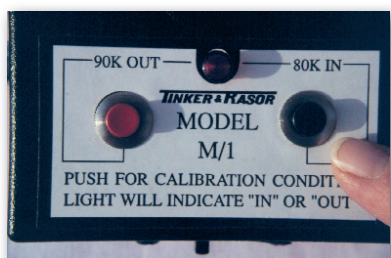
Verify detector is “IN” calibration
