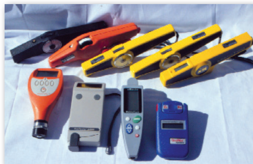
Magnetic pull-off and electronic coating thickness gages
