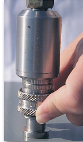
Attach quick connect locking ring to pull stub
