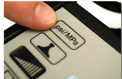
Unit of Measurement Selection Button (G)
