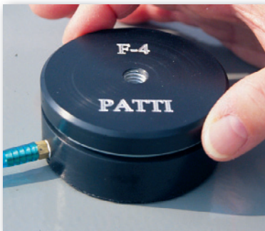
Thread top plate onto pull stub
