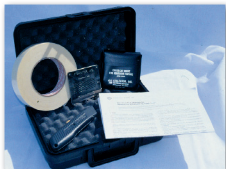
Tape adhesion test kit
