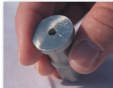
Bottom of HATE® pull stub
