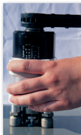
Rotate hexagon nut to increase load
