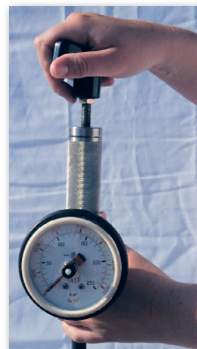
Increase pressure by turning hand lever clockwise
