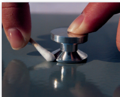
Remove excess adhesive
