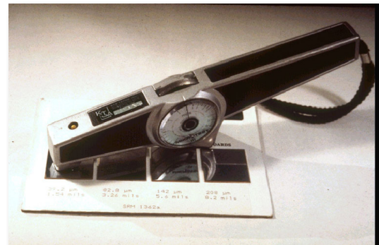
Verify the Accuracy of a Type I Gage.
