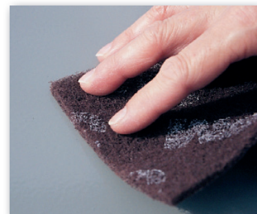
Lightly roughen surface with abrasive pad
