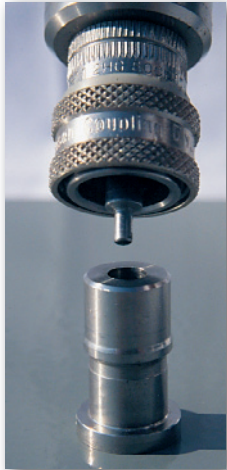
Insert pin through center hole in pull stub
