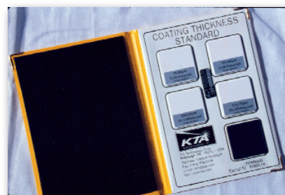
KTA coating thickness standards
