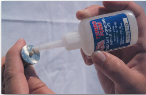
Apply adhesive to pull stub contact surface
