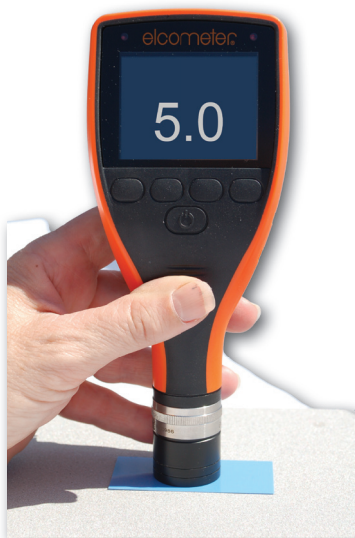
Place gage probe on low thickness shim
