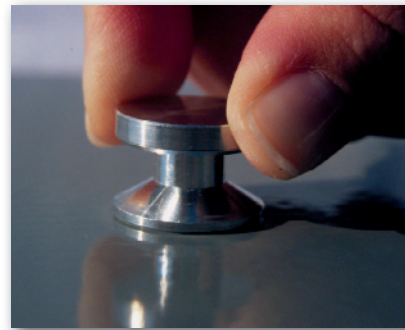
Attach pull stub
