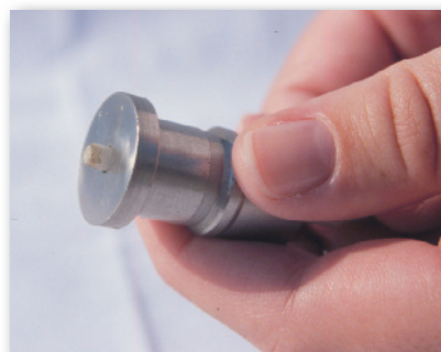
Small tip of teflon plug protrudes from bottom of HATE® pull stub
