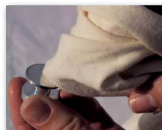
Clean pull stub
