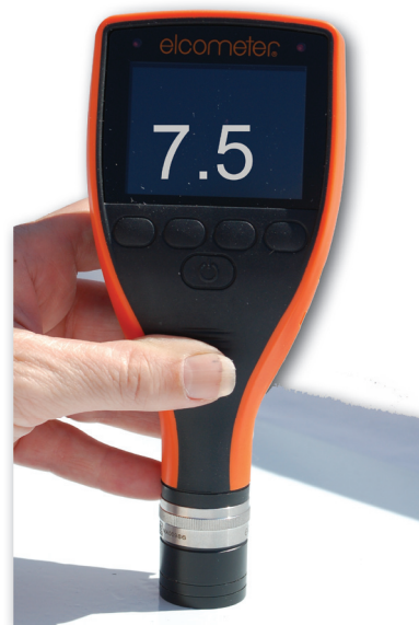
Measure the coating thickness
