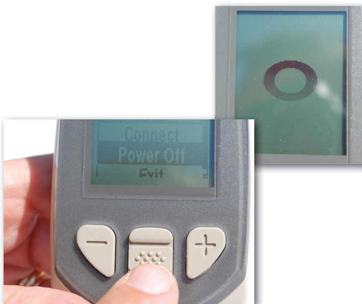
Power down gage
