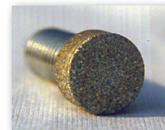
Bottom of PATTI® pull stub
