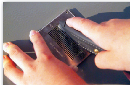
Cutting parallel incisions into coating film
