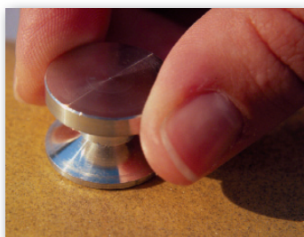
Roughen pull stub base
