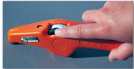
Obtain a base metal reading (BMR)
