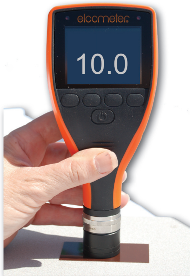
Place gage probe on high thickness shim
