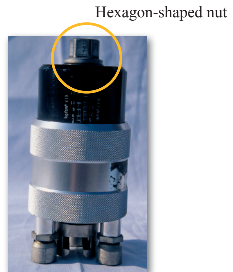
Elcometer® 106/3 or 106/4 tester (no handwheel)
