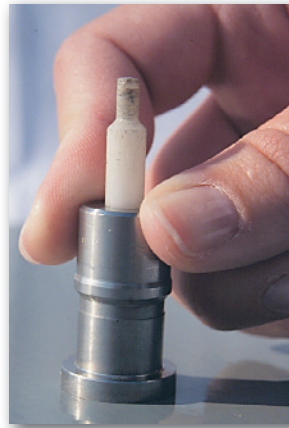
Attach pull stub to coated surface
