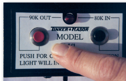
Verify detector is not “OUT” of calibration
