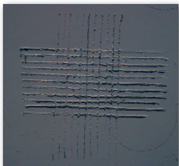
Cross-cut pattern (1mm spacing)
