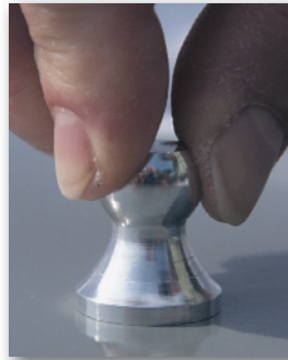
Attach pull stub to coated surface
