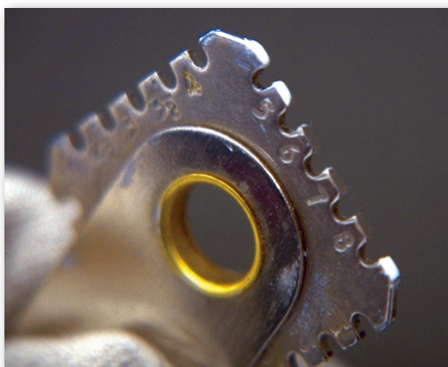
Wet film thickness of 5 mils
