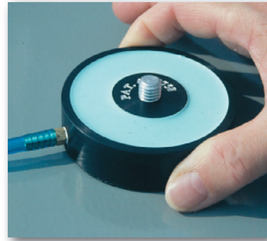
Position piston base over pull stub
