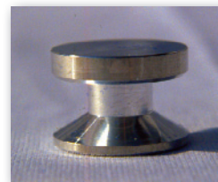
Elcometer pull stub (proper orientation)
