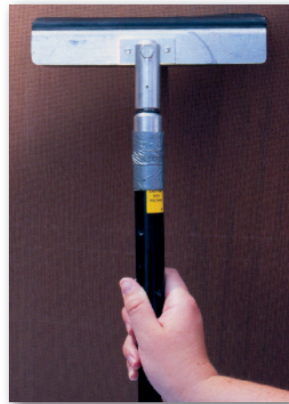
Inspect coated surfaces for pinholes/holidays
