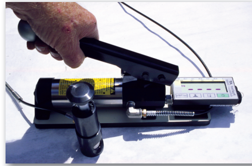
Pump lever to increase hydraulic pressure
