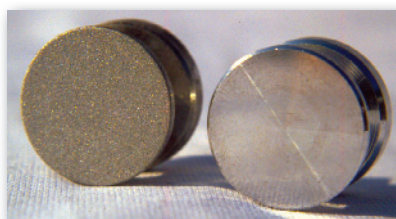
Blast cleaned (L) versus non-blast cleaned (R) pull stub
