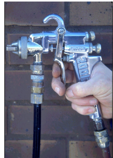
Half-Triggering a Conventional Spray Gun
