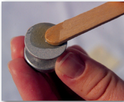
Apply adhesive to pull stub
