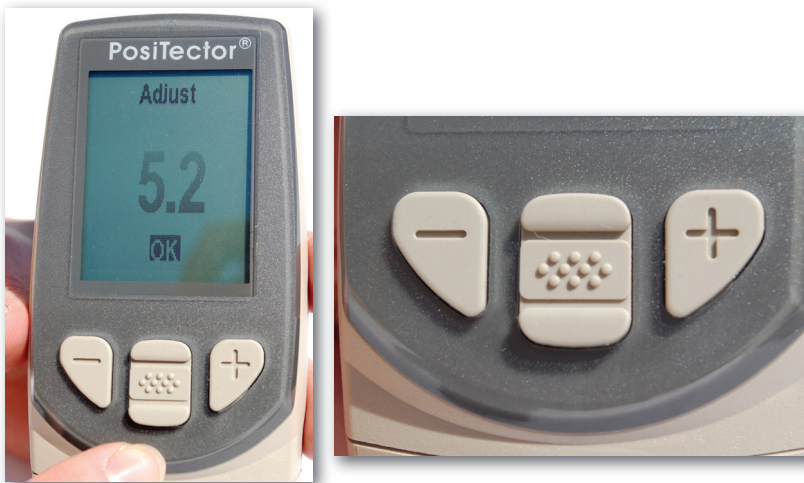
Figure 16: Adjust value to match shim thickness
