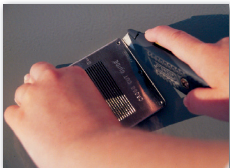
Use a straight edge to make cuts
