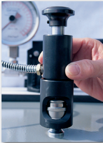
Position actuator onto pull stub
