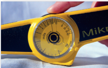
Retract scale wheel until magnet releases (↻)
