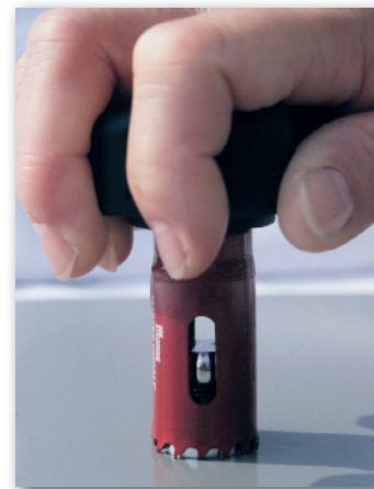
Scoring coating around perimeter of pull stub (if specified)
