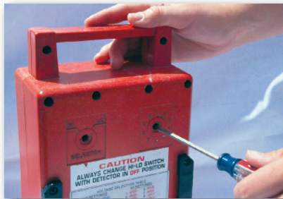
Adjust the voltage setting on the detector
