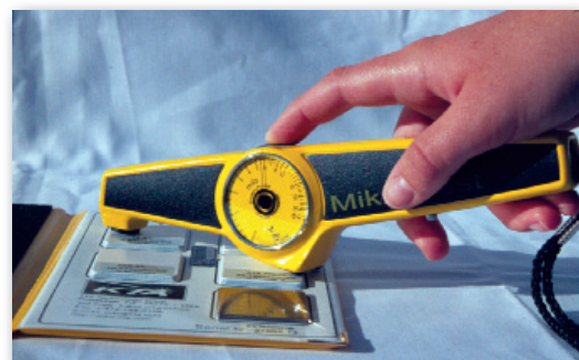
Verifying accuracy of automatic magnetic pull-off gage
