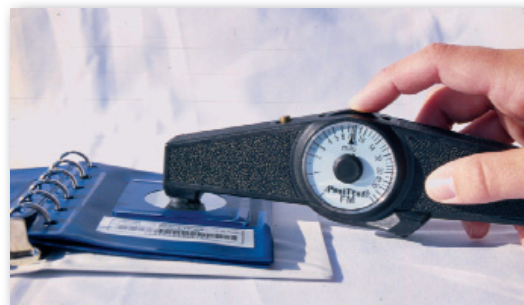
Verifying accuracy of manual magnetic pull-off gage
