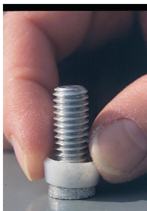
Slide plastic cut-off ring over pull stub
