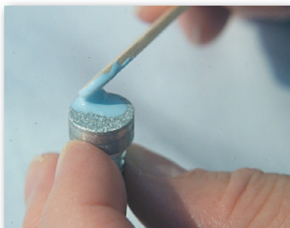
Apply adhesive to contact surface of pull stub
