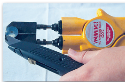
Clean contact surface of HATE® pull stub using heat clamp and knife blade
