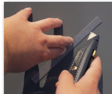
Cutting incision into coating film
