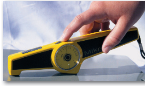
Rotate scale wheel forward first (↺)
