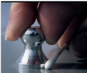
Remove excess adhesive
