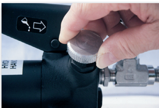
Open pressure release valve
