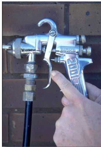
Half-Triggering a Conventional Spray Gun
