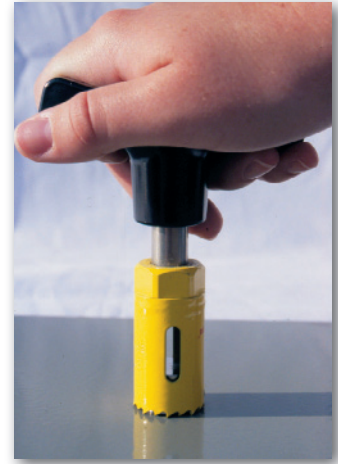
Scoring the coating (if specified)
