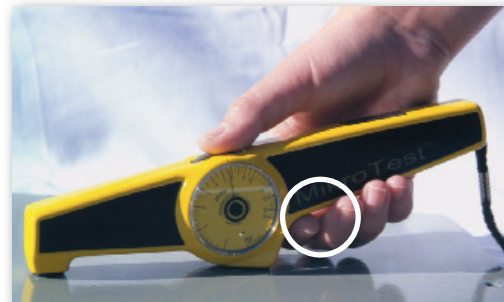
Rotate scale wheel forward, then push in counter weight button (↻)
