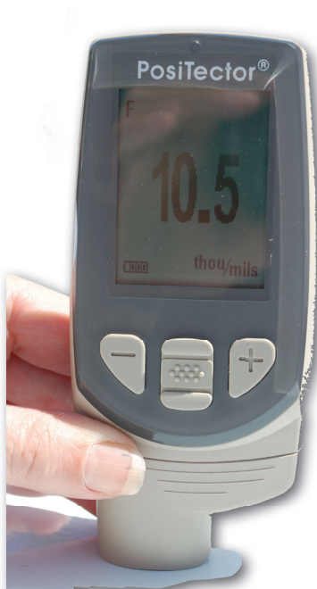
Measure the coating thickness
