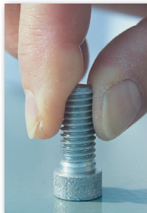
Attach pull stub to coated surface
