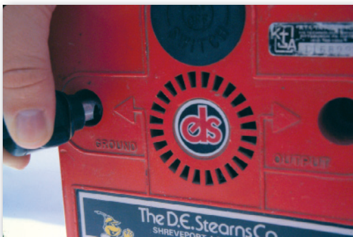
Insert ground wire connector into detector port “GROUND”
