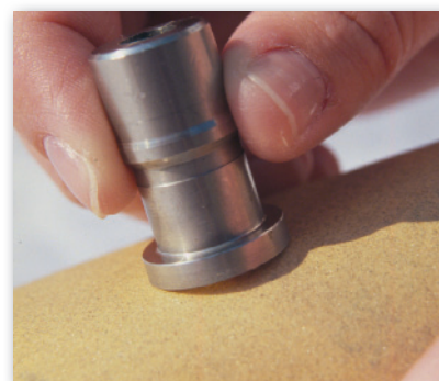
Roughen pull stub contact surface
