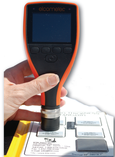
Verification of accuracy using coating thickness standards (need to measure and subtract BMR)
