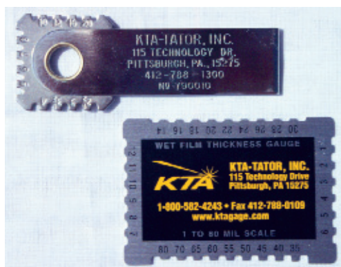
Stainless steel and aluminum notch-type WFT gages
