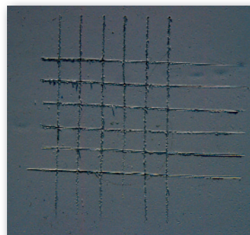
Cross-cut pattern (5mm spacing)
