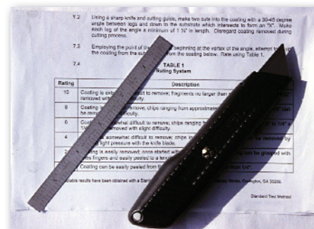
Knife, ruler, and test method
