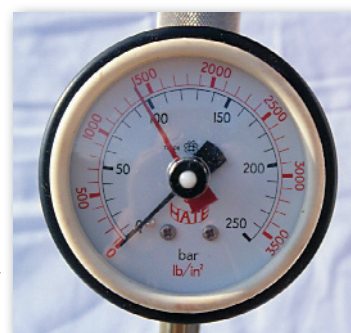
Read red sweep needle (1,400 psi shown)
