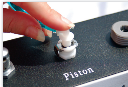
Connect blue air hose to piston port
