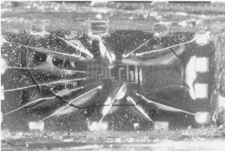
Figure 5.1. Integrated circuit showing wire breakage due to shrinkage stresses after coating with a silicone varnish.
