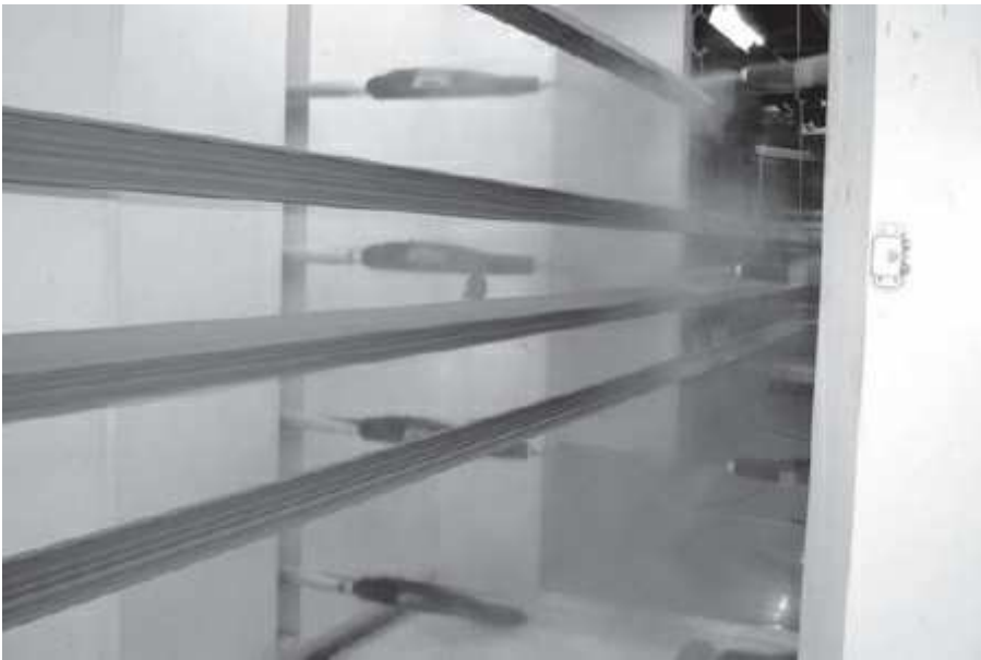
Figure 8.3: Electrostatic spray equipment
