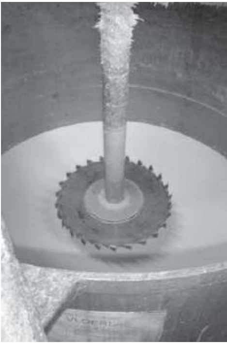
Figure 7.9: Dispersing tank with high-speed serrated-edge disk
