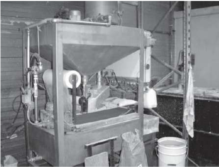
Figure 10.1: Water cleaning machine with flocculate agent and filtration cloth
