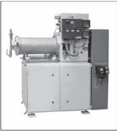
Figure 7.11: Horizontal pearl mill disperser, source: Bühler, Switzerland
