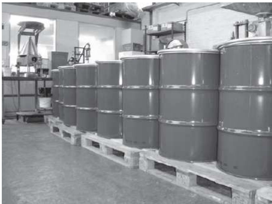
Figure 7.1: 200 litre vessels used for binders and solvents
