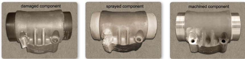
Fig. 9.17 Restoration process of a mechanically damaged flap transmission tee box housing of an aircraft via CSAM [40]
