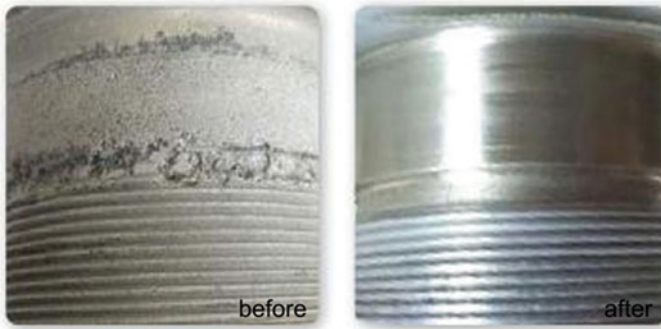
Fig. 9.16 Restored B737 nose wheel steering actuator barrel via CSAM [40]
