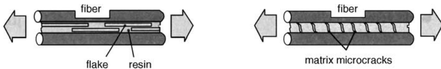
Figure 3.17 Cross Section with and without Mica
