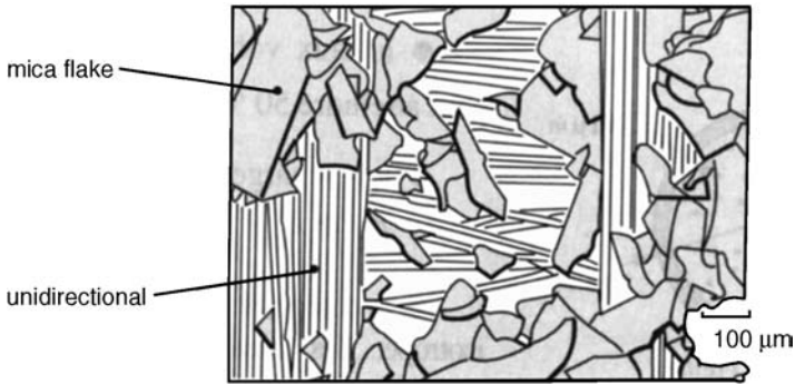
Figure 3.16 Mica Flakes Arrangement
