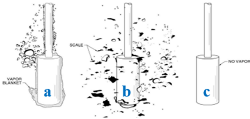
Figure 8.32. Different stages of quenching: (a) vapor-blanket stage, (b) vapor transport cooling stage and (c) liquid cooling stage.
