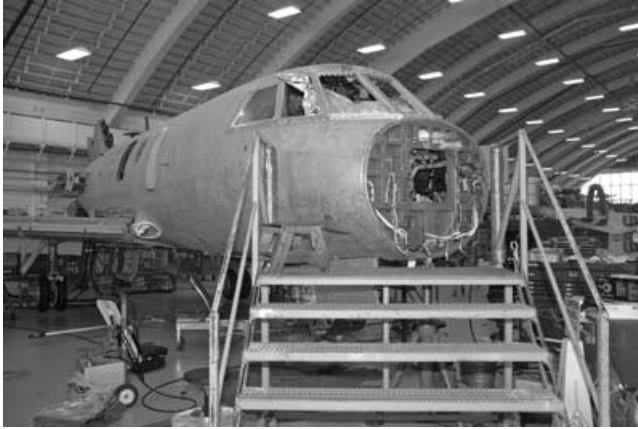
1.1 A Dassault Falcon jet undergoing corrosion inspection and repair. Manufactured in 1983 and designed as a corporate business jet, this aircraft flies low-altitude maritime search-and-rescue missions in a corrosive marine environment. The aircraft is scheduled to retire in 2021.
