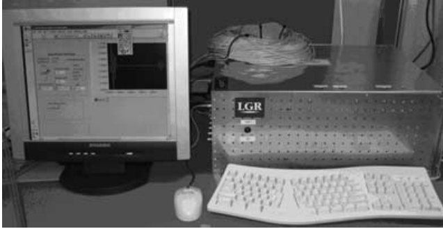
7.7 LGR's lock-in based FBG interrogation prototype system.
