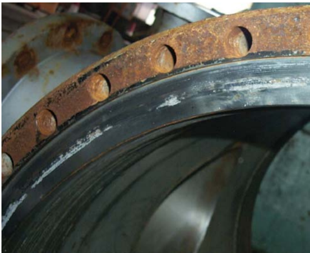
Figure 3.6 Photograph of a part of heat-exchanger sheet affected by crevice corrosion. The carbon steel shell was weld-cladded with SAF 2507 alloy. Note, only the gasket area of the shell suffered from attack; shell side was exposed to seawater. (Source: Raja (2008). Reproduced with permission of Narosa Publishing House.)
