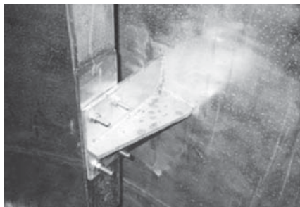
Case 68 (a) Corrosion pits on a baffle support bracket and nearby areas on the shell. (b) Corrosion pits on the shell above the weld line.
