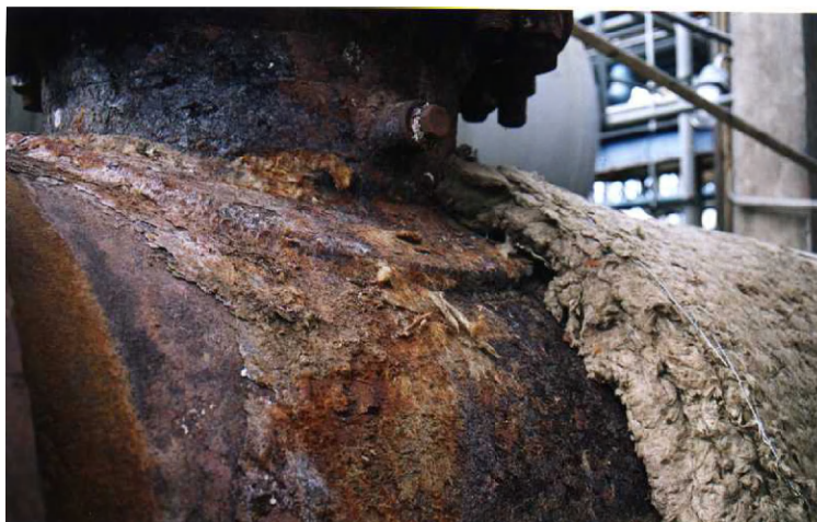
Fig. 3.9 Corrosion of a heat exchanger under thermal insulation. (For a full color version of this figure, see the Color Section)
