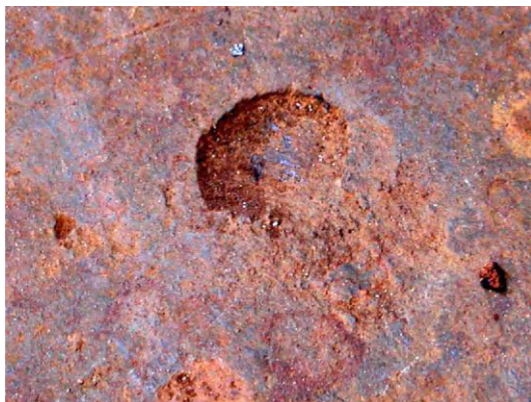
Fig. 2.10 MIC on a metal surface compared with pitting, crevice, differential aeration cell, or galvanic corrosion. The bottom of a crude oil storage tank after a microbial attack. (For a full color version of this figure, see the Color Section)
