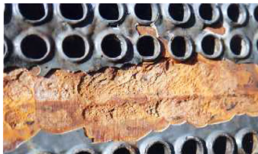
Fig. 2.9 Galvanic corrosion of coated carbon steel tube sheet because of high ratio between cathode (Admiralty brass tubes) and anode area (carbon steel tube sheet coated with epoxy). Gray – failed epoxy coating; yellow – rusted tube sheet. (For a full color version of this figure, see the Color Section)
