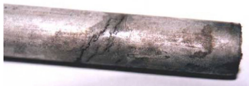
Fig. 2.17 Chloride stress corrosion cracking of an SS 316 tube in the atmosphere containing HCl gas.
