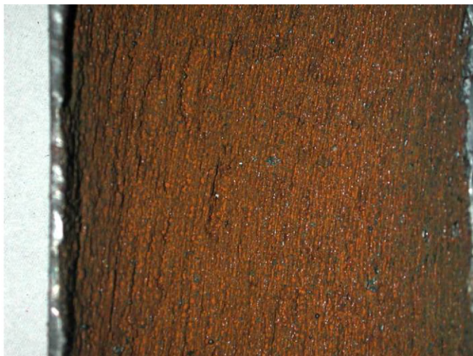
Fig. 2.16 Erosion-corrosion inside a liquefied petroleum gas (LPG) carbon steel tube. “Grooves” are formed as a result of erosion. (For a full color version of this figure, see the Color Section)
