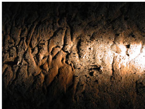
Fig. 3.17 Corroded bottom of a crude oil AST. The morphology of the surface and microbiological examination showed MIC. (For a full color version of this figure, see the Color Section)
