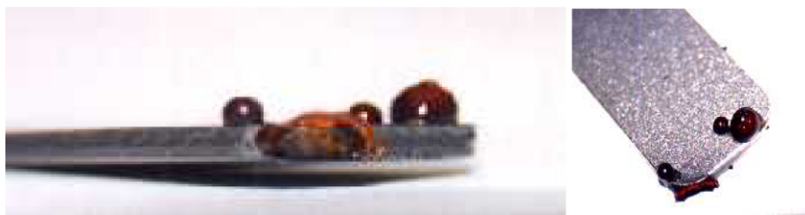
Fig. 3.11 Corrosion "balls" formed on a carbon steel surface (strip coupons) after 3 days' immersion in kerosene with water (1 wt %) added. (For a full color version of this figure, see the Color Section)
