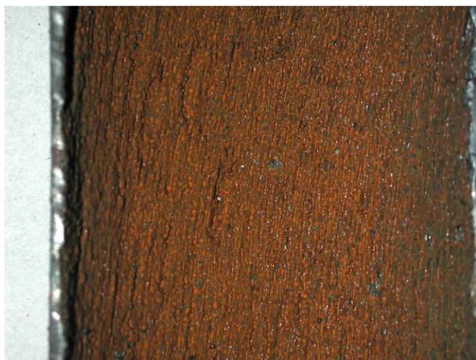
Fig. 2.16 Erosion-corrosion inside a liquefied petroleum gas (LPG) carbon steel tube. “Grooves” are formed as a result of erosion.
