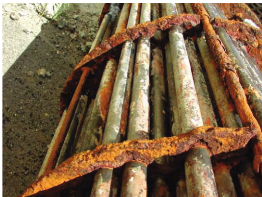
Fig. 2.6 Heat exchanger: tubes made of titanium and baffles made of carbon steel (cooling water, 4 years). Deposits on the titanium tubes are the salts (scale) formed from the cooling water, and not corrosion products. (For a full color version of this figure, see the Color Section)
