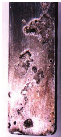
Fig. 2.4 Under deposit corrosion : corrosion pits formed under \text{NH}_4\text{Cl} acidic salt deposits on a carbon steel surface (4 months).
