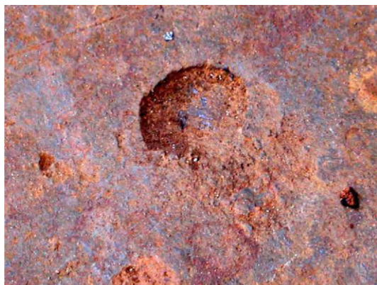
Fig. 2.10 MIC on a metal surface compared with pitting, crevice, differential aeration cell, or galvanic corrosion. The bottom of a crude oil storage tank after a microbial attack.
