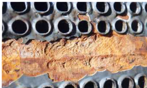
Fig. 2.9 Galvanic corrosion of coated carbon steel tube sheet because of high ratio between cathode (Admiralty brass tubes) and anode area (carbon steel tube sheet coated with epoxy). Gray – failed epoxy coating; yellow – rusted tube sheet.
