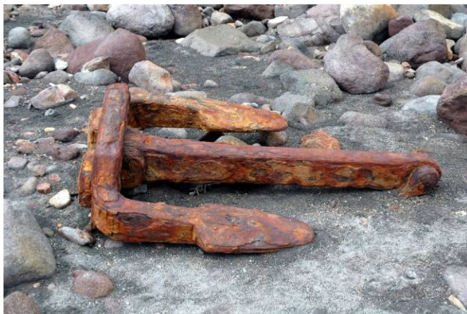
Fig. 1.12 Corroded anchor made of carbon steel.
