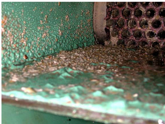
Fig. 3.2 Scale (calcium and magnesium carbonates) formed inside of heat exchanger with cooling water after 4 years. (For a full color version of this figure, see the Color Section)
