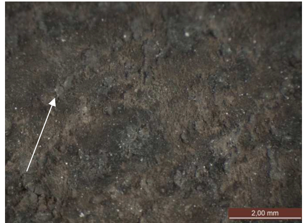
Fig. 5 Detail of the corrosion layer with a network of minute cracks at the site marked with an arrow
