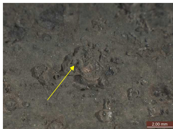
Fig. 9 Detailed picture of the inner surface of pipe 3 with tubercles
