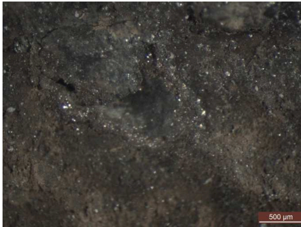
Fig. 4 Corrosion layer deposited on inner surface of pipe 2
