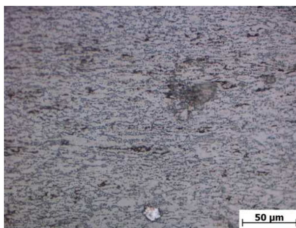
Fig. 1 Microstructure of tested Ti6Al4V alloy, etch. 10 ml HF, 5 ml HNO 3 and 85 ml H 2 O
