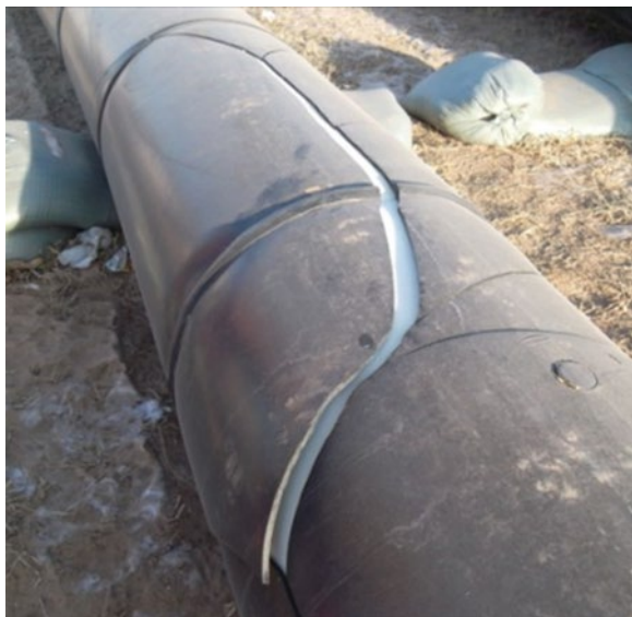
Figure 9.2 Completely disbonded three-layer PP coatings removed from a gas pipeline (see colour plate section).
