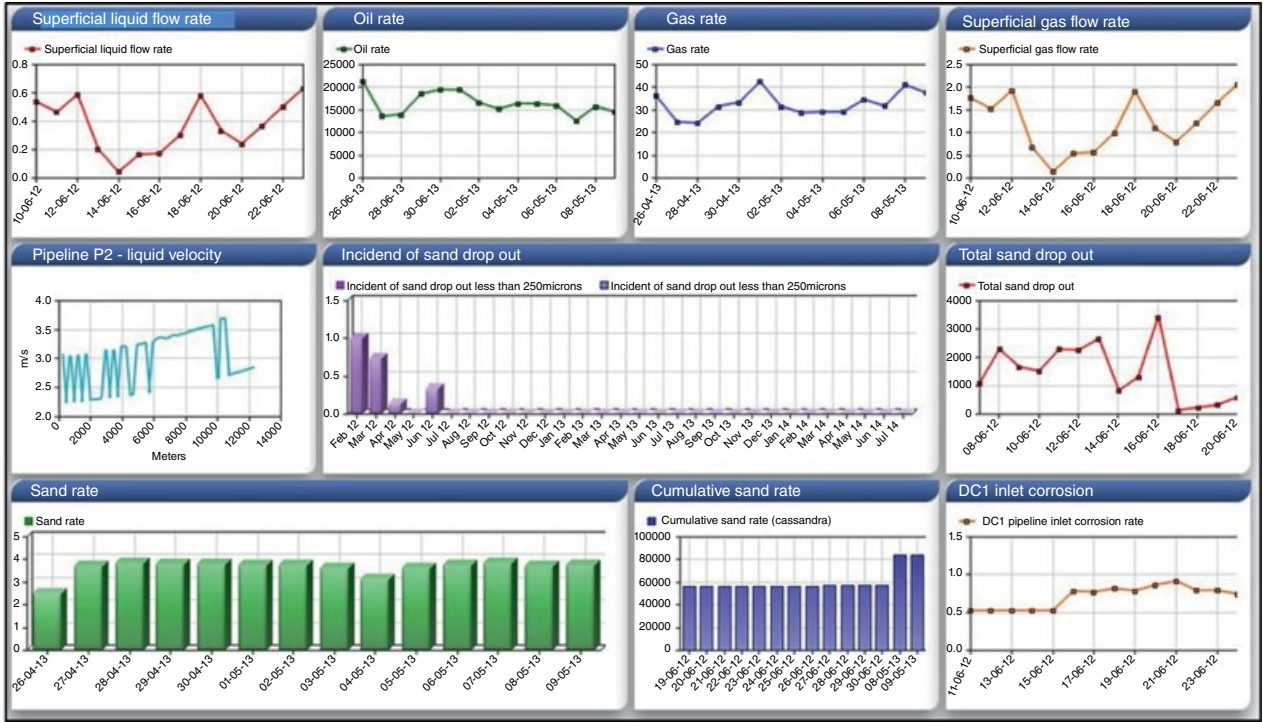
Figure 10.4 An example of a corrosion management dashboard.
