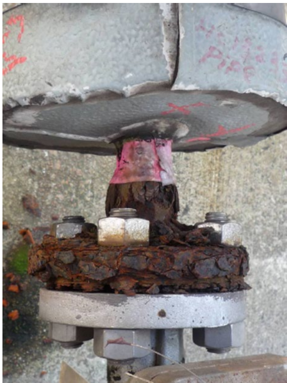
Figure 13.6 A typical example of carbon steel sweating CUI damage accelerated by galvanic corrosion at a carbon steel/stainless steel flange material specification change. (see colour plate section).
