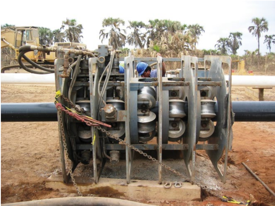
Figure 15.4 An example of roller box reduction equipment.
