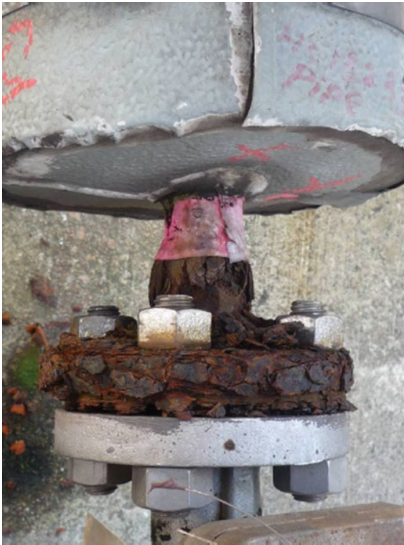
Figure 13.6 A typical example of carbon steel sweating CUI damage accelerated by galvanic corrosion at a carbon steel/stainless steel flange material specification change.
