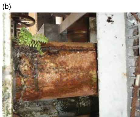
Figure 13.1 (a) and (b) typical examples of CUI showing devastating consequence of the corrosion threat.
