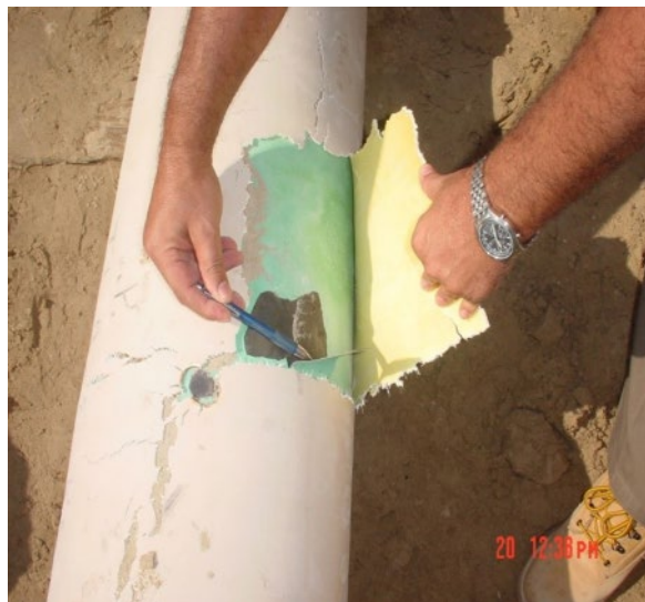
Figure 9.3 Cracking and disbondment of the three-layer PP coating due to thermo-oxidative degradation. (see colour plate section).
