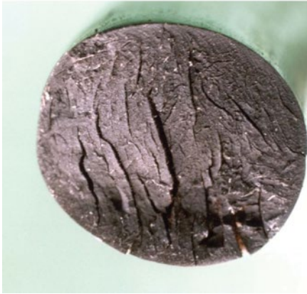
Figure 15.3 Examples of decompression damage to rubber.
