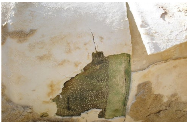
Figure 9.4 Failure of a flame-sprayed PP field joint coating on a three-layer PP-coated gas pipeline.
