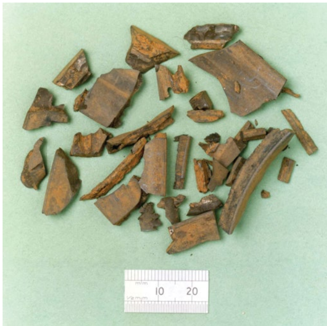
Figure 15.1 An example of heat ageing of a rubber seal.
