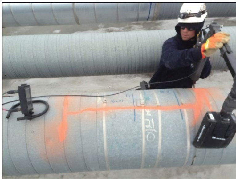
Figure 10.5 A one-person-operated, portable RT unit in use.
