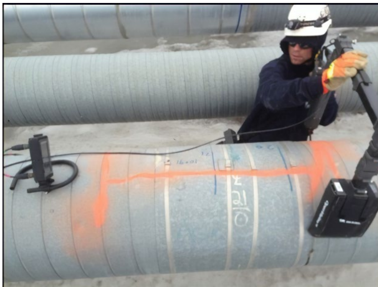
Figure 10.5 A one-person-operated, portable RT unit in use. (see colour plate section).
