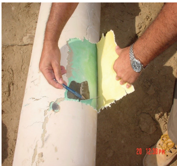
Figure 9.3 Cracking and disbondment of the three-layer PP coating due to thermo-oxidative degradation.
