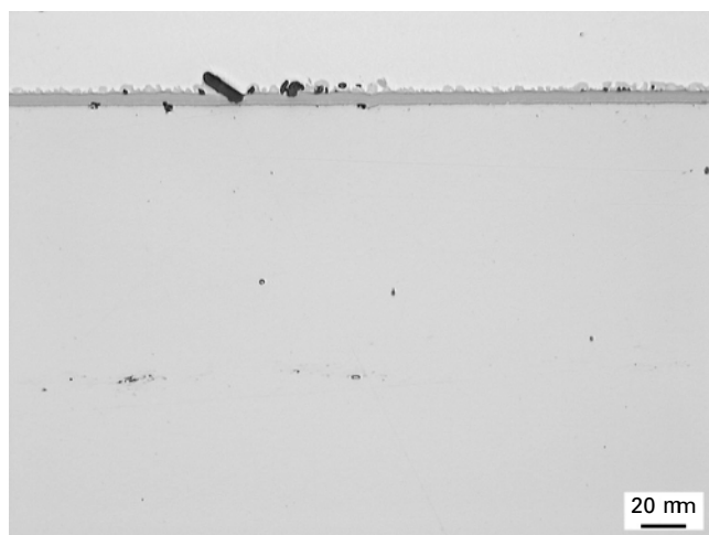
7.8 Ti-carbide layer as a result of the Ti-Al co-diffusion coating process on Alloy 10CrMo9 10.
