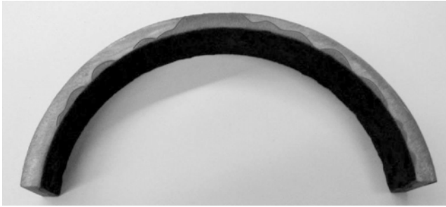
15.8 Cross-section of a pyrolysis tube with (patchy) carburized areas.
