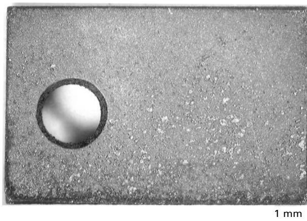
7.23 Alloy P91 coated with a Si-Ti-Al co-diffusion coating tested at 620°C under industrial atmosphere for 1345 h. Formation of a protective oxide scale on the surface.
