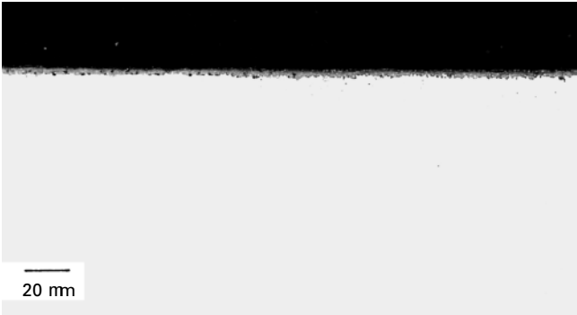
8.5 Thin chromia scale on Cr-5%Fe-1%Y 2 O 3 after 10000h under metal dusting conditions at 650°C.
