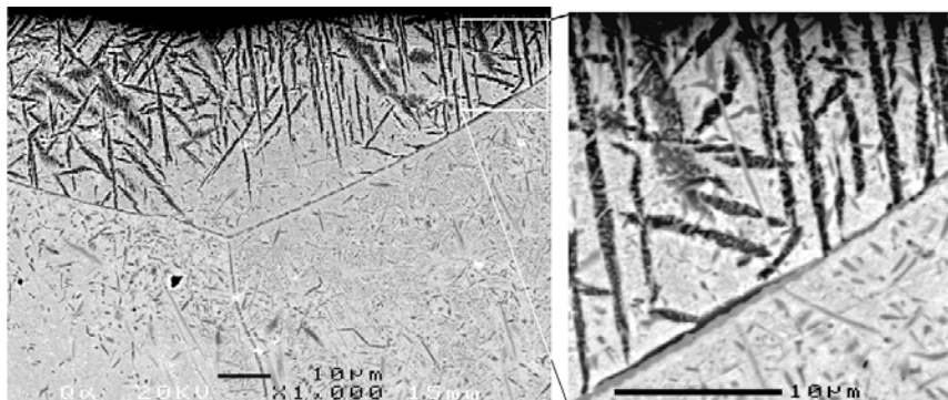
13.6 FeCrAl alloy exposed in a metal dusting environment for 5000 h. SEM cross-section of the reaction front in bottom of a metal dusting pit. Light grey in contrast are M_7C_3 carbides, dark in contrast are possibly k-carbide ( M_3AlC ) with strong orientational growth in the ferritic lattice.
