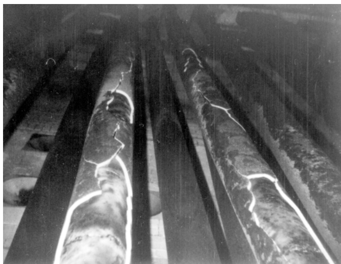
15.2 Typical brittle failure of a radiant tube in a pyrolysis coil.
