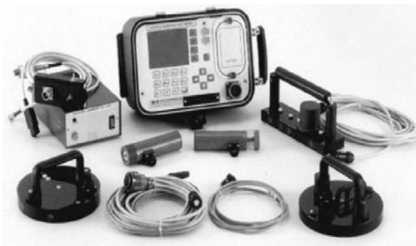
Figure 4.17 Gecor 8 (developed from Gecor 6 Figure 4.13) has separate heads for corrosion rate of atmospherically and buried or submerged corrosion rate measurement, resistivity, and assessment of cathodically protected structures. Courtesy James Instruments and Geocisa.
