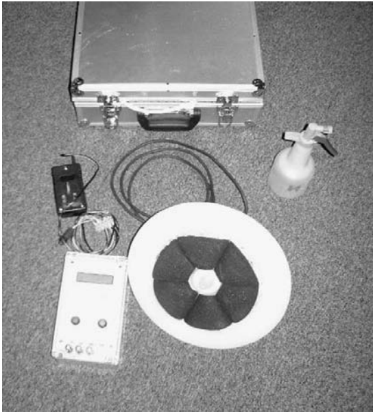
Figure 4.16 BGB Bigfoot LPR probe with manual meter and charger. A 'little foot' probe is also available for accessing small spaces such as concrete rafters under floor boards.
