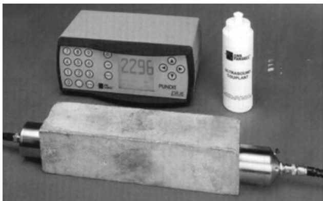
Figure 4.24 The Pundit Plus system for use in direct transmission mode. Courtesy CNS Farnell Ltd.
