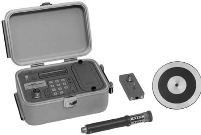
Figure 4.13 The Gecor 6 linear polarization meter with sensor controlled guard ring for corrosion rate measurement (circular sensor A) and concrete cover resistance/resistivity head (tubular sensor B). Courtesy James Instruments USA and Geocisa SA, Spain.
