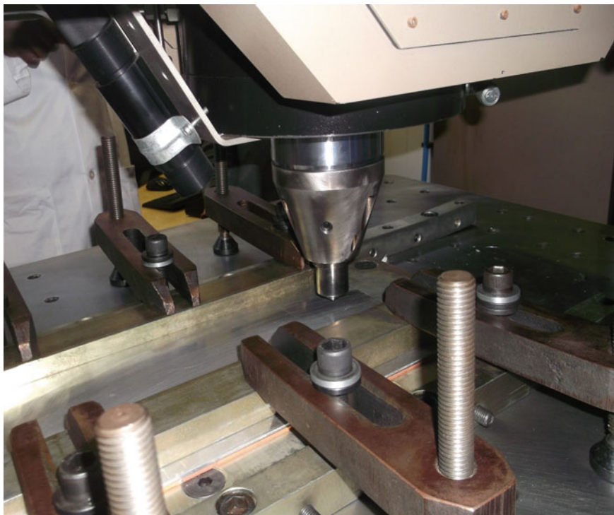
Fig. 4.1 Shows the MTS PDS I-Stir used to produce the friction stir spot welds
