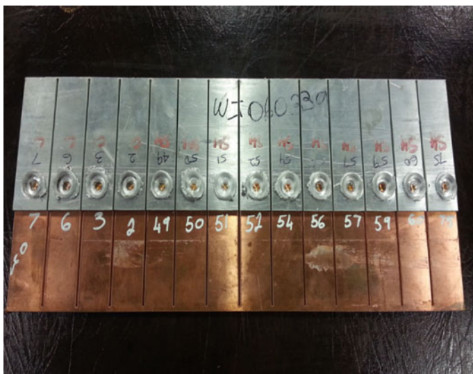
Fig. 5.4 Shows some of the specimens used for the shear tensile test in the current study
