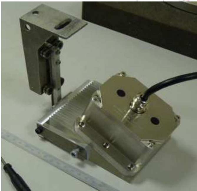
Figure 83 The 2D-1 array on its Rexolite wedge of 18.5° designed to generate longitudinal waves in the component.
