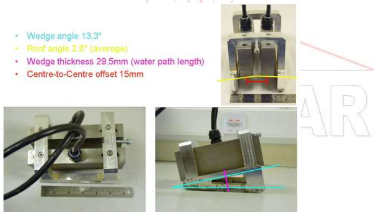
Figure 82 The final configuration of the TRL-1 probe, ready to be used for inspection.
