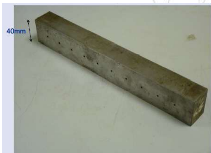
Figure 179 The reference carbon steel calibration block containing target SDHs and dimensions similar to the coupon extracted from the weld (see Figure 175).
