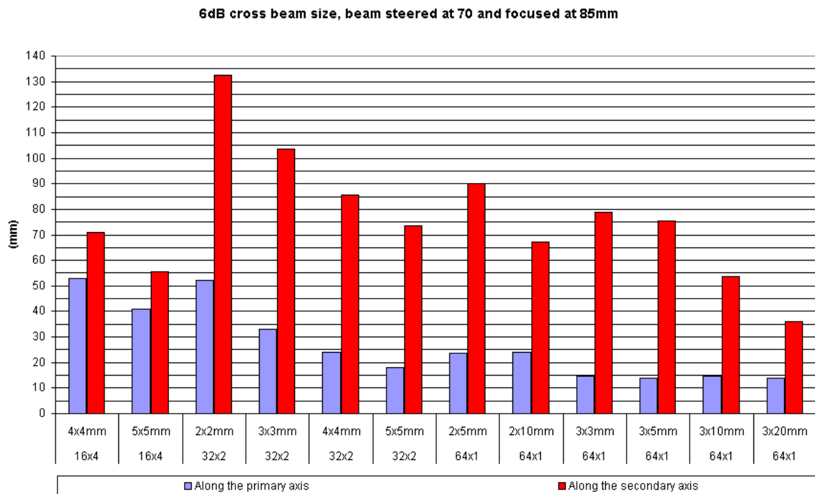
Figure 55 The -6dB cross beam measurement from the SimulUS models for all 12 cases.
