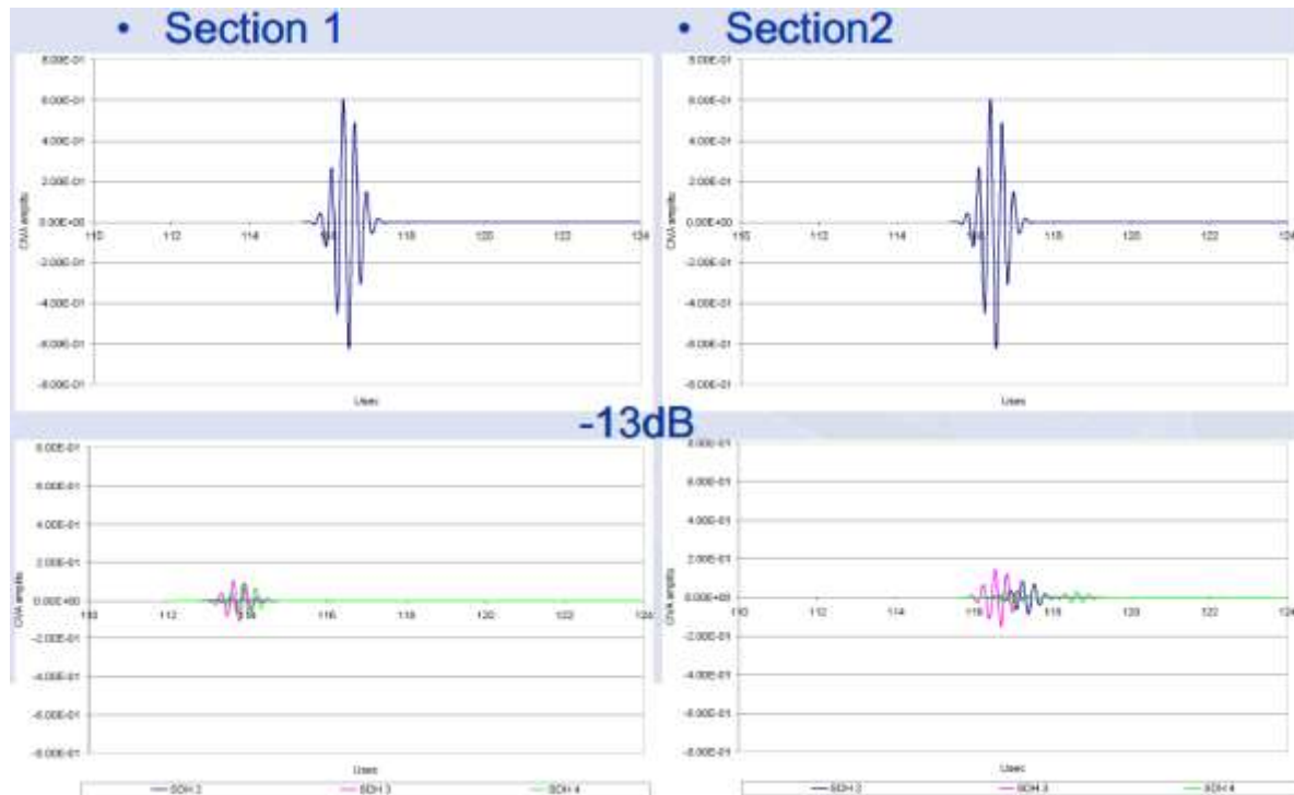
Figure 185 Simulated signals from the SDHs in the carbon steel (top) and the validation block (bottom) for the two different weld sections.
