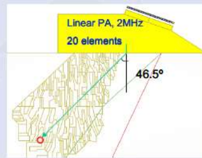
Figure 145 Two possible approaches to generate ADLs through simulation: using the expected flaw itself (left) or using a generic SDH in the correction region of the weld (right).
