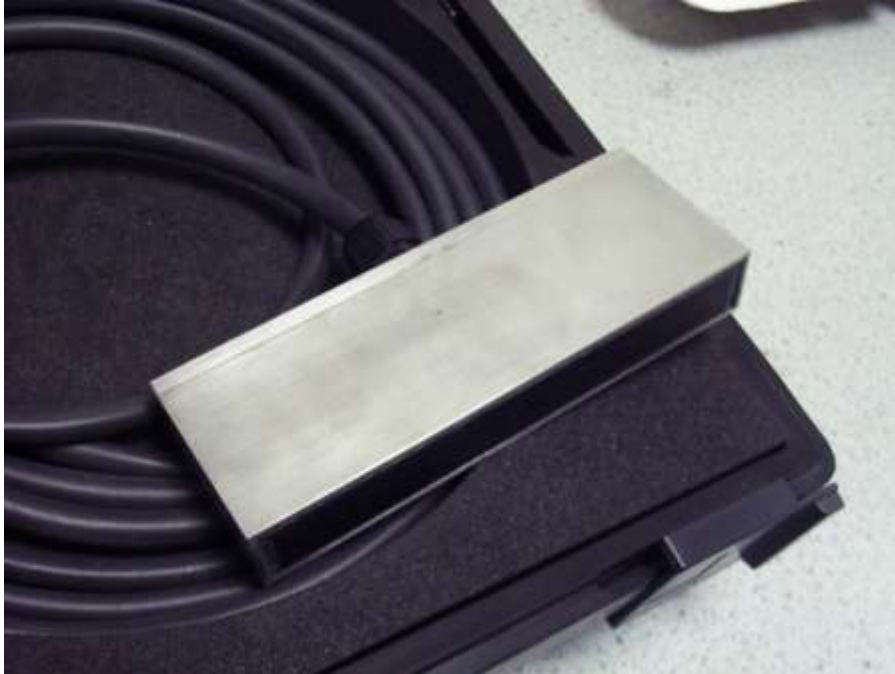
Figure 76 A half of the TRL-1 array, as received after manufacture.
