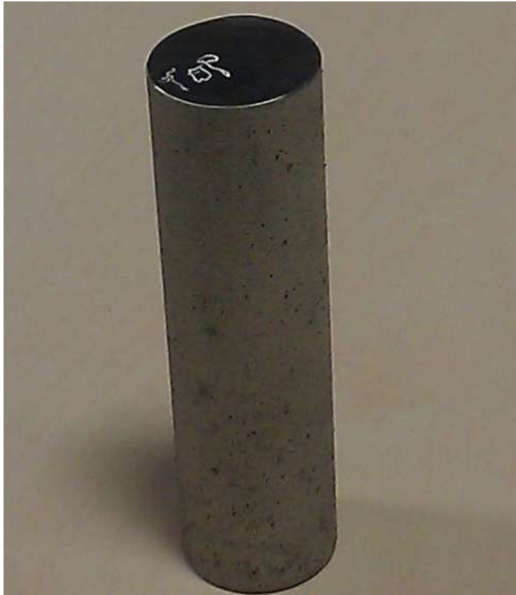
Figure 176 The Inconel alloy single crystal cylinder (20mm diameter, 70mm length) grown for the validation of the model in the DISSIMILAR project.
