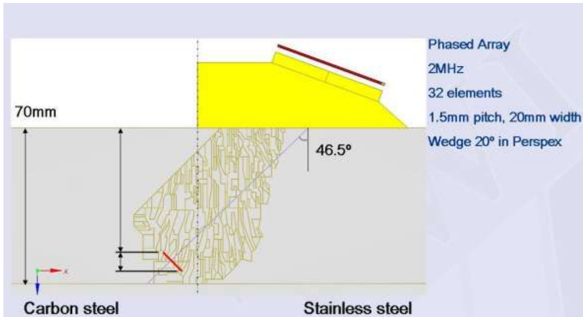
Figure 90 The inspection scenario for a specular incidence inspection of Flaw 3.
