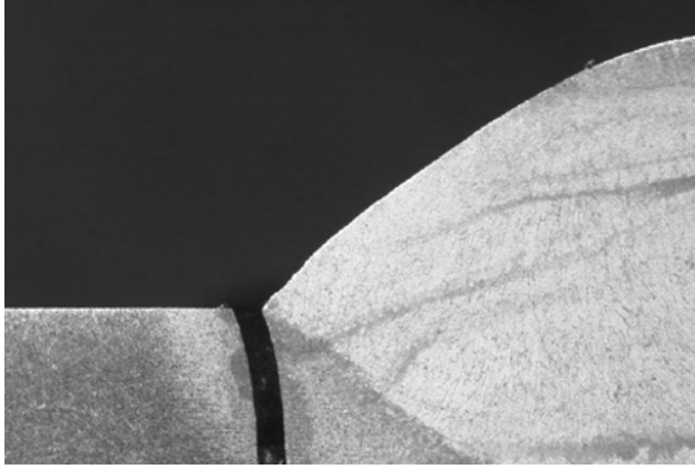
Figure 7.1 Typical location of a fatigue crack
