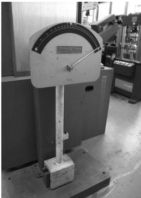
Figure 7.2 Impact test machine for assessing toughness
