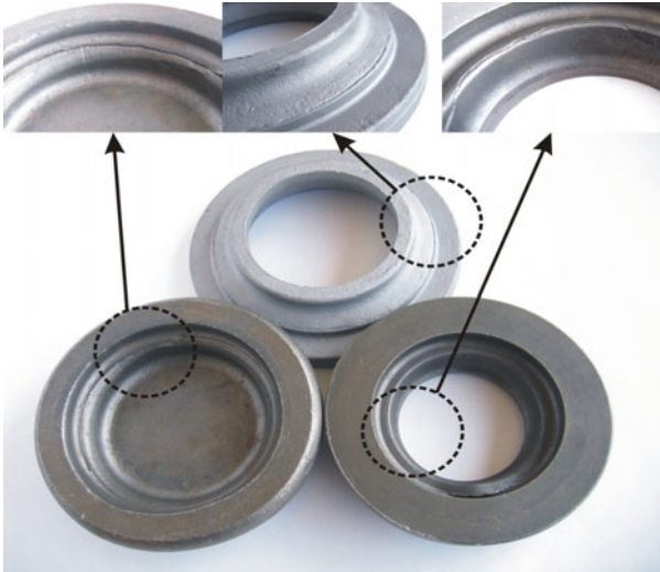
(a) Some axisymmetrically flanged parts in macro-scale with folding defects.
