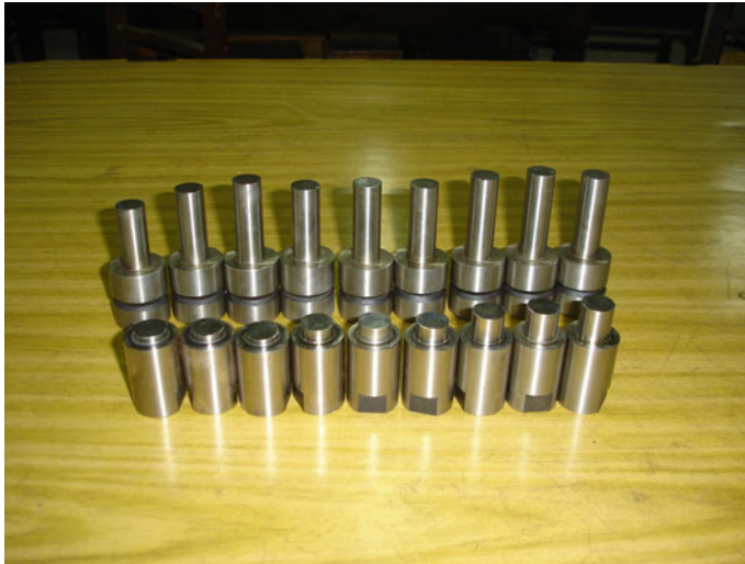
Fig. 3.5 Different punches and die inserts fabricated for forming different designed parts
