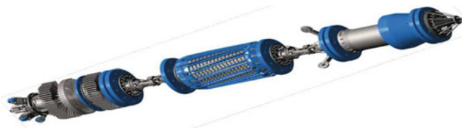
Fig. 3.10 Combined tool of two types: MFL and UT CD (image taken from the website: http://www.transneft.ru )
