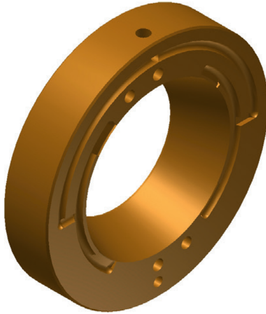
Figure 11.10 Face of striping ring for 4 stripes
