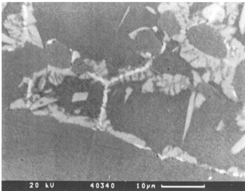
3.19 Backscattered SEM micrograph of grey \sigma - and white \chi -phases. Steel S32750 after 900°C for 10 minutes, \times 2000 .
