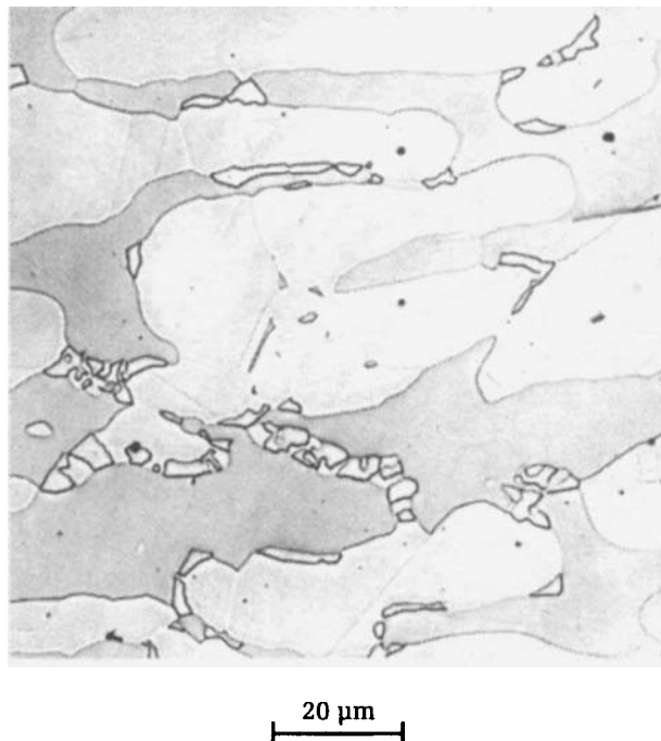
3.17 Coarse sigma precipitates in superduplex plate after 10 minutes at 1000°C, \times 800 . Etch: electrolytic sulphuric acid.
