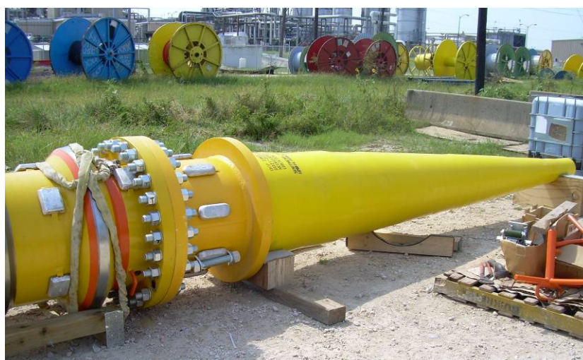
Figure 22 Typical umbilical bend stiffener
