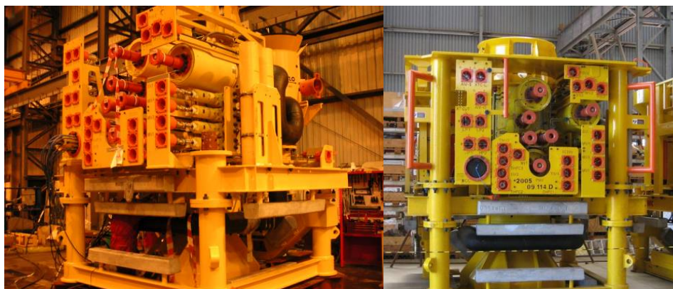
Figure 5 Typical subsea tree assemblies
