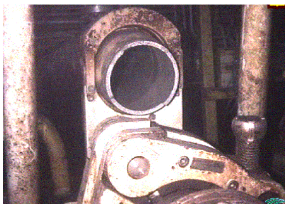
Figure 24 Full bore fracture of superduplex stainless steel manifold hub connector
