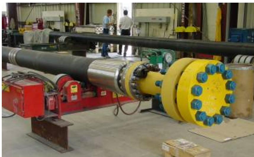
Figure 18 Titanium alloy taper stress joint for deep water steel catenary riser application
