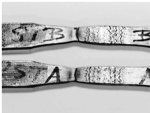
Figure 2-9. Tensile Specimens (2) for Test Plate NS-4, 1/2-in. (455/STT)
