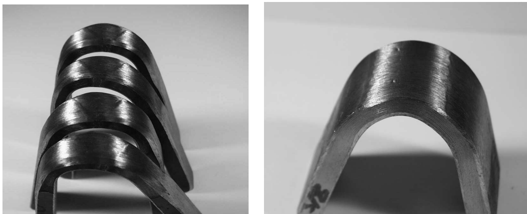
Figure 2-2. Side Bends (4) and Face Bend (1) for Test Plate N-1, 5/8-in. (455/STT)
