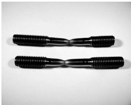
Figure 2-3. Tensile Specimens (2) for Test Plate N-1, 5/8-in. (455/STT)
