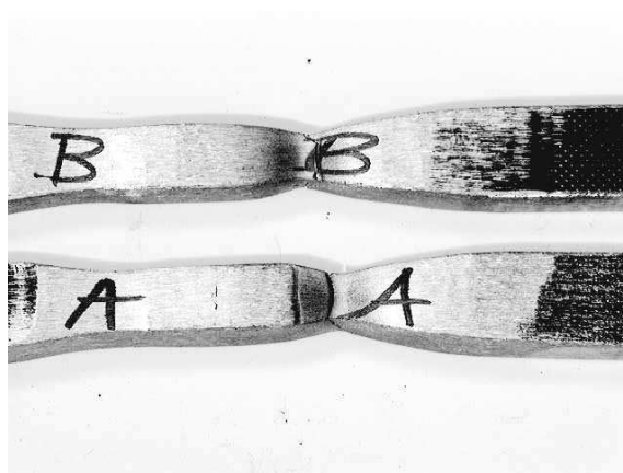
Figure 2-5. Tensile Specimens (2) for Test Plate N-2, 3/4-in. (455/STT)
