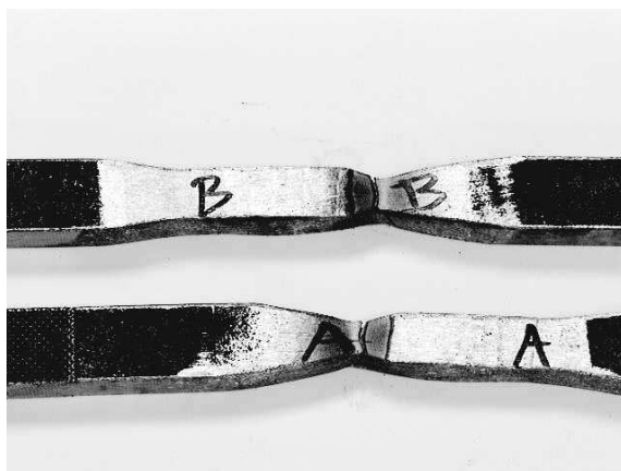
Figure 2-7. Tensile Specimens (2) for Test Plate N-3, 1-in. (455/STT)
