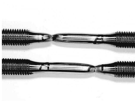
Figure 2-11. Tensile Specimens (2) for Test Plate N-5, 3/4-in. (455/STT)
