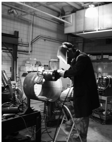
Figure 3-1. Demonstration of open root V-groove (5G Position).
