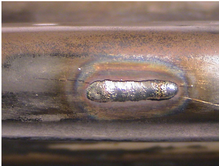
Figure 5-8 Typical Failure Location After Cycling
