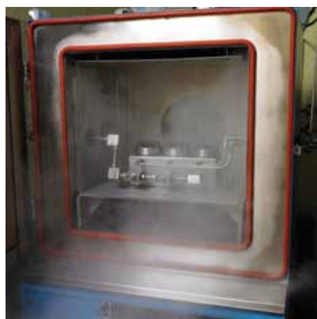
Figure 35: Low temperature environment chamber for testing sealing on static 'O' rings.
