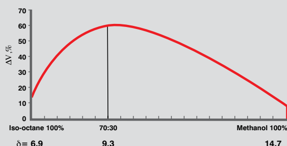
Figure 40: Variation of volume swell for low ACN nitrile in blends of iso-octane:methanol.
