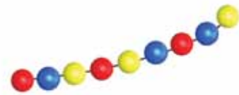
Figure 5: Three different monomers form a terpolymer.
