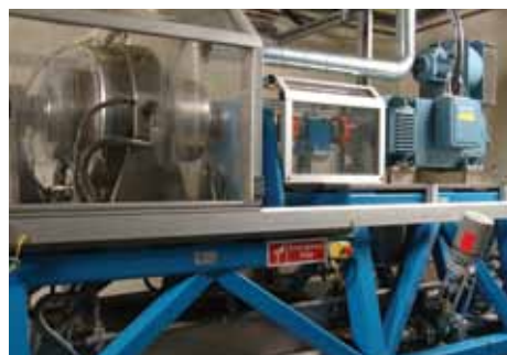
Figure 36: Example of bespoke test equipment for evaluating a rotary cartridge assembly.
