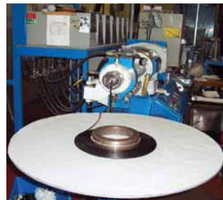
Figure 17: Screw extruder producing extrusion for the manufacture of 'O' rings.
