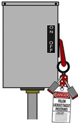
Figure 4.8 A multiple lock device is signed by each person who affixes a lock.
