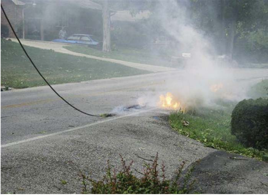
Figure 8.8 Downed power lines that are still energized can spark and cause fires. It is easy to tell that this line is still energized.
