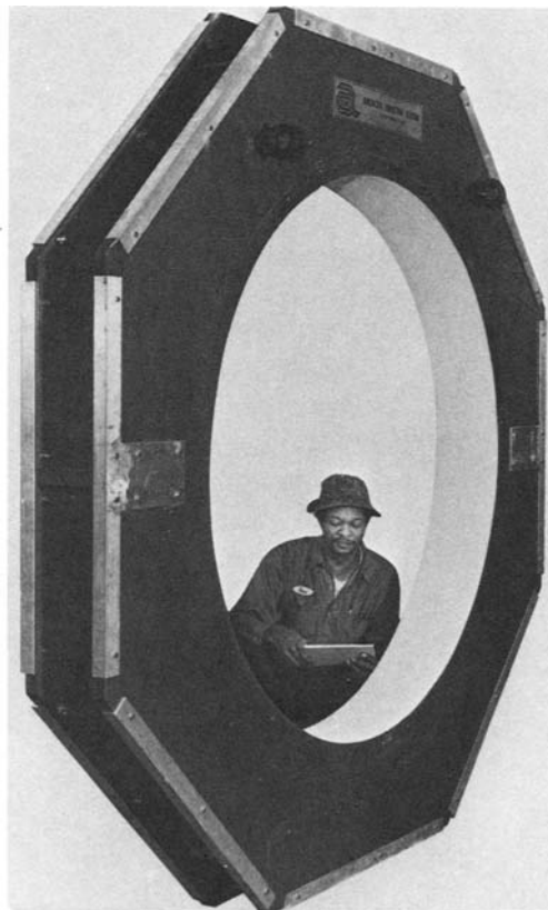
Fig. 11.8. Induction heating arrangement used to strip 152-cm (60-in.) printing rolls (source: American Induction Heating Corp.)
