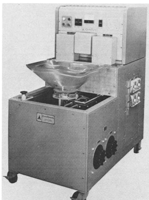
Fig. 11.21. Photograph of a getter flashing system used in production of television tubes (source: Lindberg Cycle-Dyne, Inc.)
